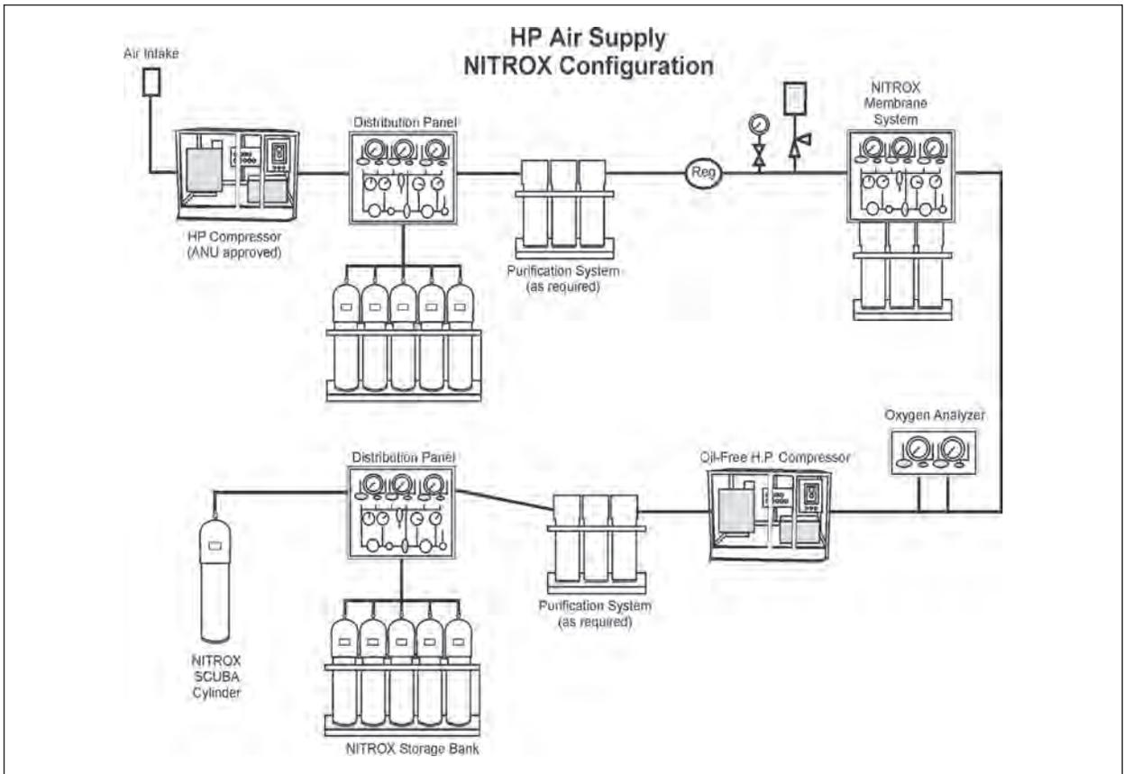
**Figure 10-5.** HP Air Supply NITROX Membrane Configuration.
