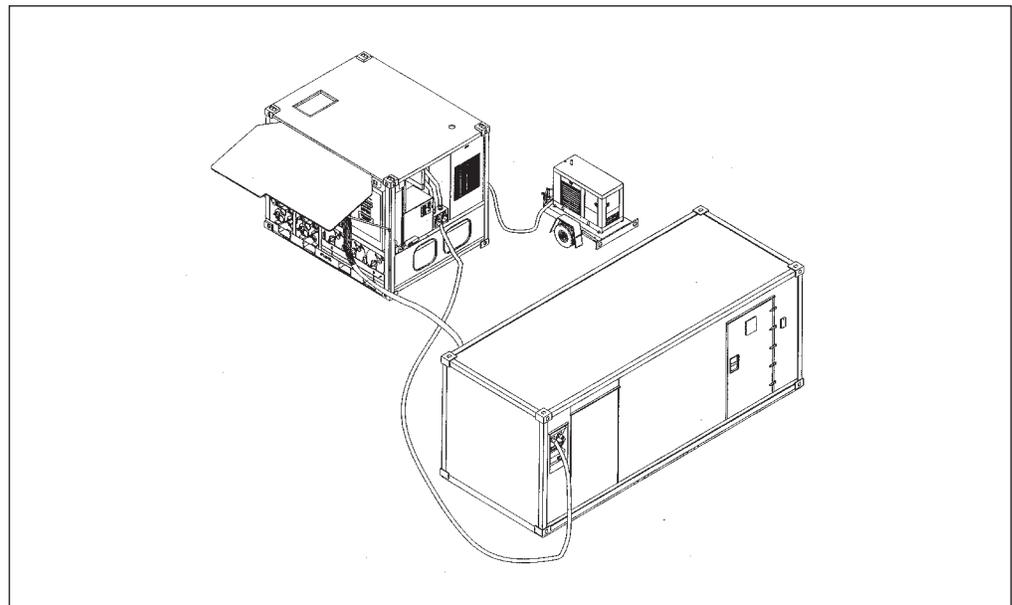
**Figure 18-10.** Fly Away Recompression Chamber (FARCC).
