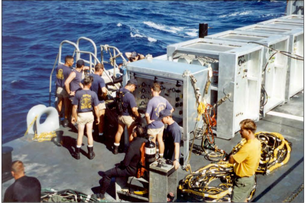
Figure 12-1. FADS III Mixed Gas System (FMGS).
