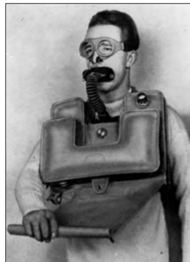
**Figure 1-10.** Original Davis Submerged Escape Apparatus.
