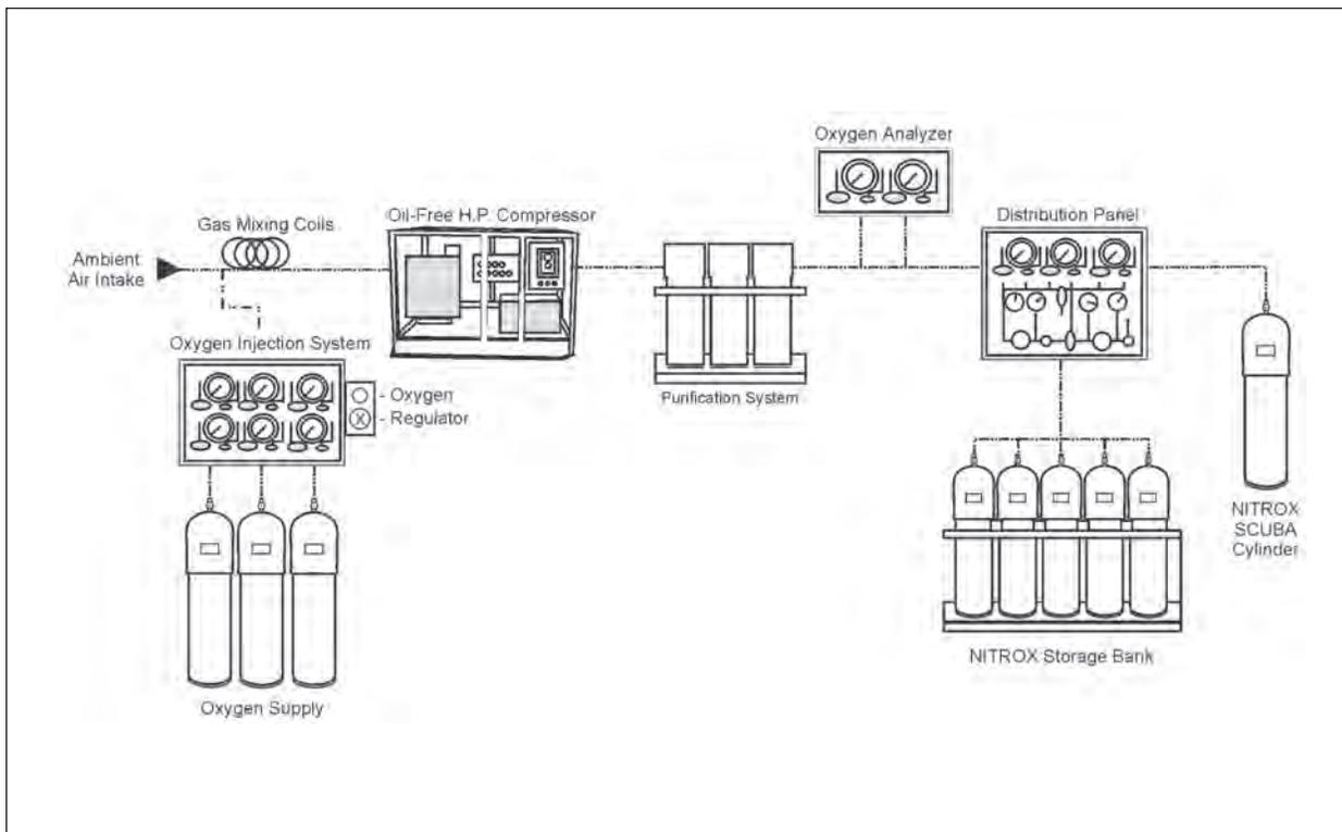
Figure 10-3. NITROX O<sub>2</sub> Injection System.
