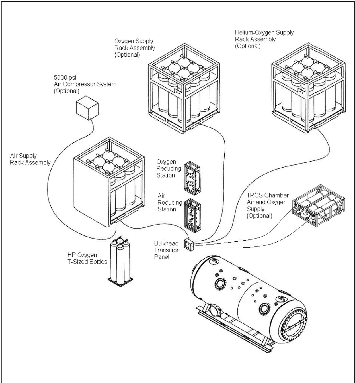
**Figure 18-6.** Standard Navy Double-Lock Recompression Chamber System.
