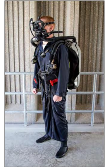
**Figure 15-1.** MK 16 MOD 1 Closed Circuit Mixed Gas UBA.
