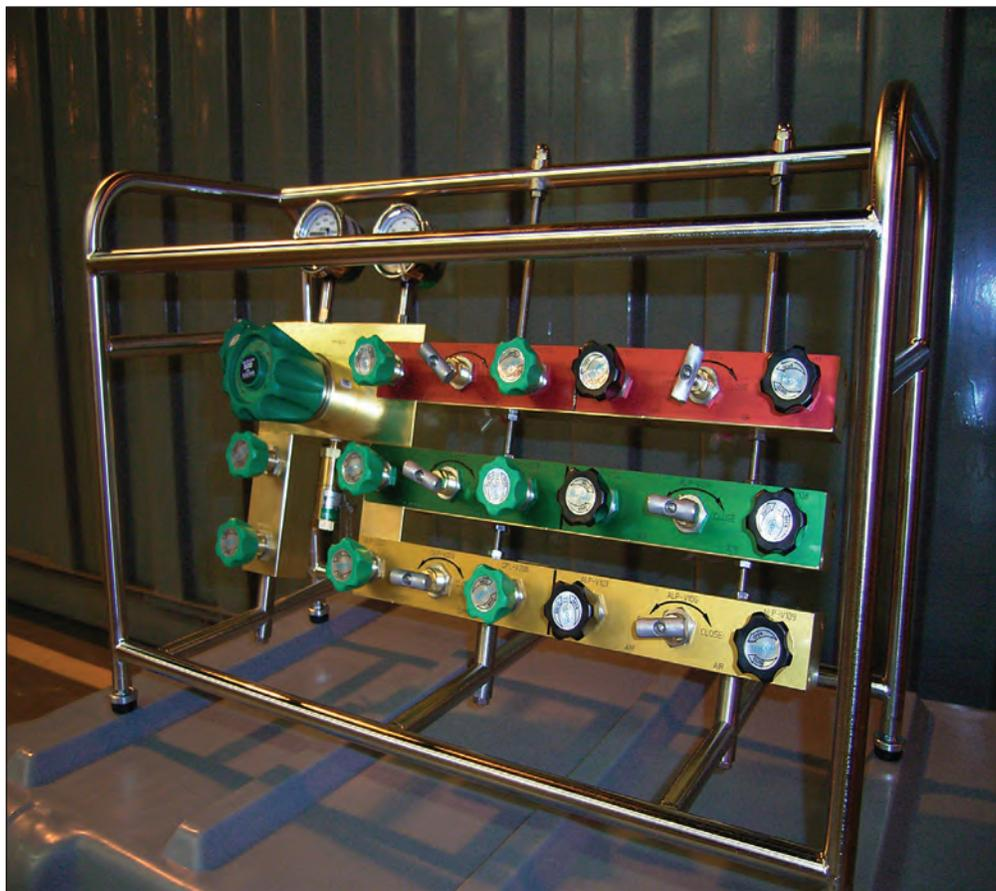
**Figure 8-10.** Oxygen Regulator Control Assembly (ORCA) II.
