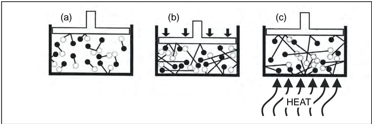
**Figure 2-6.** Kinetic Energy. The kinetic energy of the molecules inside the container (a) produces a constant pressure on the internal surfaces. As the container volume is decreased (b), the molecules per unit volume (density) increase and so does the pressure. As the energy level of the molecules increases from the addition of thermal energy (heat), so does the pressure (c).
