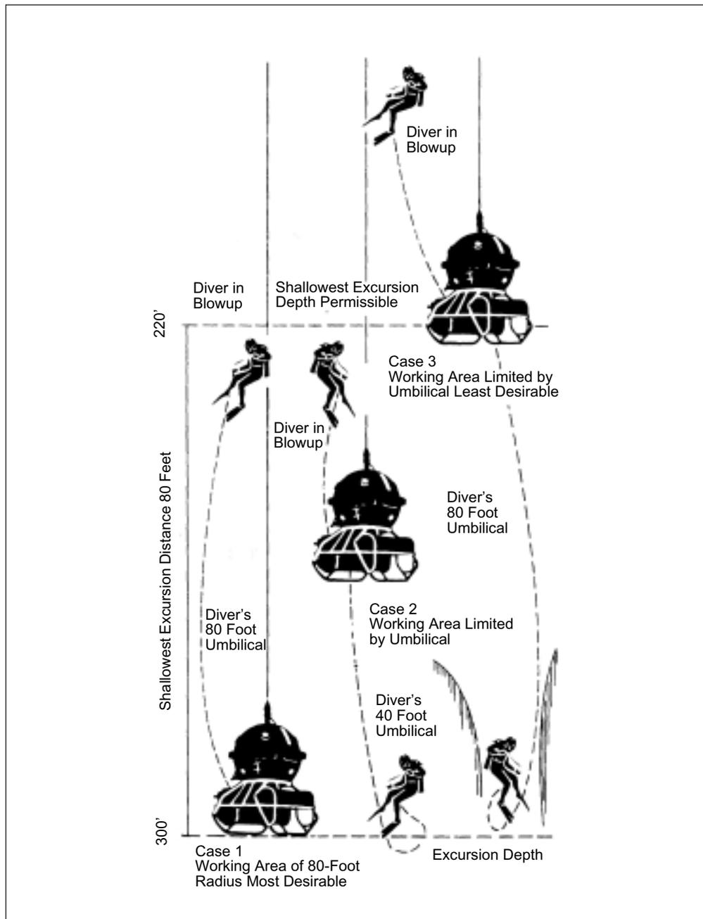
Figure 13-12. PTC Placement Relative to Excursion Limits.
