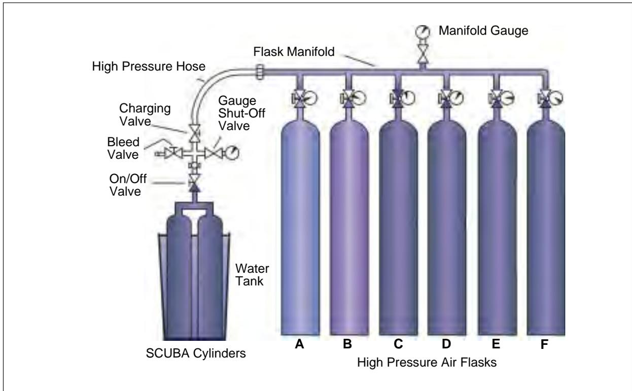
**Figure 7-9.** Cascading System for Charging SCUBA Cylinders.
