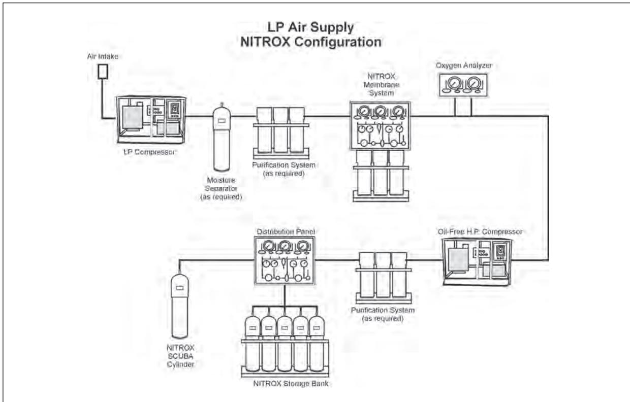
Figure 10-4. LP Air Supply NITROX Membrane Configuration.
