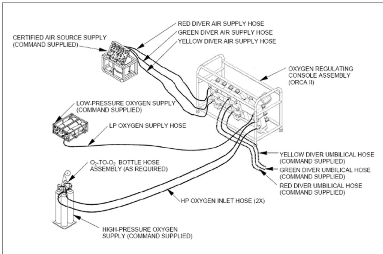
Figure 8-11. Oxygen Regulator Control Assembly (ORCA) II Schematic.
