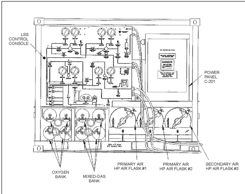
Figure 18-12. Fly Away Recompression Chamber Life Support Skid.
