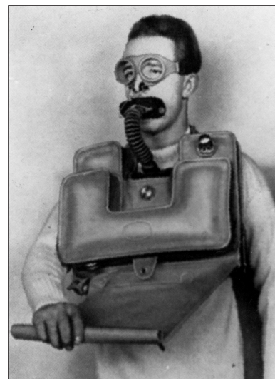
Figure 1-10. Original Davis Submerged Escape Apparatus.
