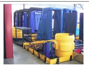
FIGURE C-3 Yellow Containment Barrel and Diver's Umbilical with Berm and DECON Deck Grating
