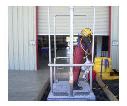
FIGURE C-2 4' X 9' X 9" Diver's Stage Berm with DECON Deck Grating
