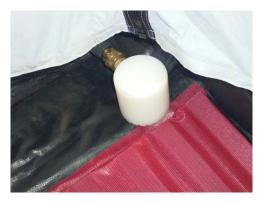
FIGURE C-13 Zumro DECON Tent Dewatering Strainer (inside)
