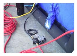
FIGURE C-12 Zumro DECON Tent Dewatering 110V Electric Pump and Hoses
