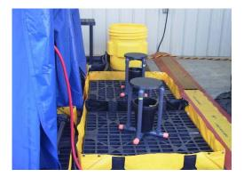
FIGURE C-6 Diver Undress Area. Table for Helmet DECON and Yellow Container for Dive Suit and Clothing. Berm, Seats, and DECON Deck Grating (privacy curtain not shown)
