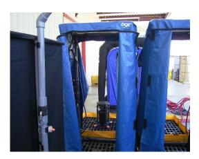
FIGURE C-5 Rinse Showers with Yellow Berm and DECON Deck Grating
