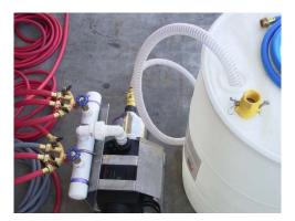
FIGURE C-8 110V Electric Water Supply Pump with manifold, shut-off valves, with suction hose and red supply hoses to showers. White 50 gal clean water supply container
