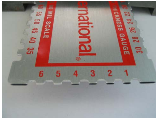
Figure 5. WFT Gauge Showing a Reading of 4-5 Mils.
