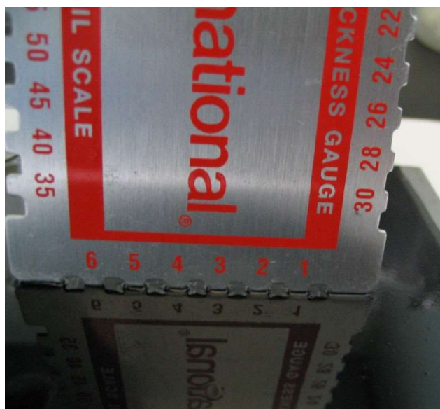
Figure 4. WFT Gauge Positioned in Wet Paint Film.
