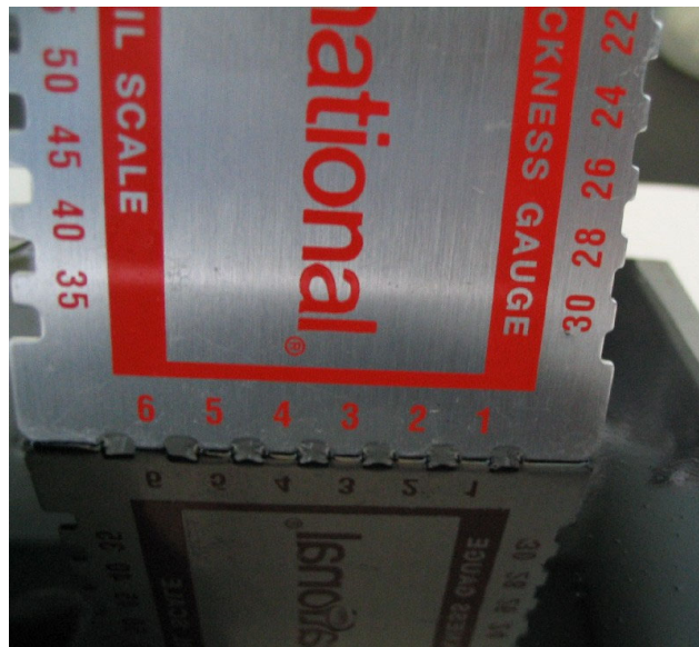
Figure 4. WFT Gauge Positioned in Wet Paint Film.
