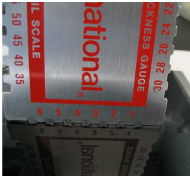
Figure 4. WFT Gauge Positioned in Wet Paint Film.
