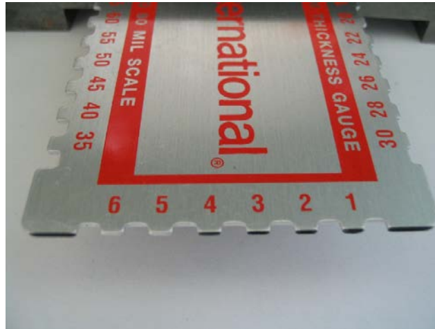
Figure 5. WFT Gauge Showing a Reading of 4-5 Mils.
