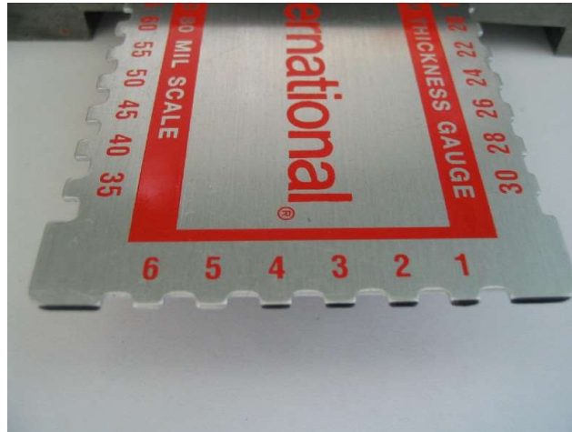
Figure 5. WFT Gauge Showing a Reading of 4-5 Mils.
