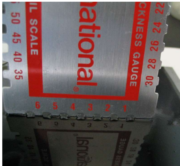
Figure 4. WFT Gauge Positioned in Wet Paint Film.
