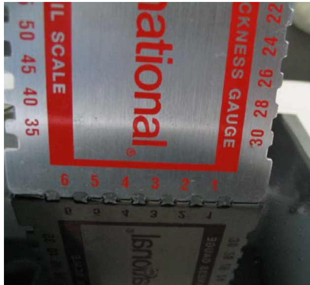
Figure 4. WFT Gauge Positioned in Wet Paint Film.
