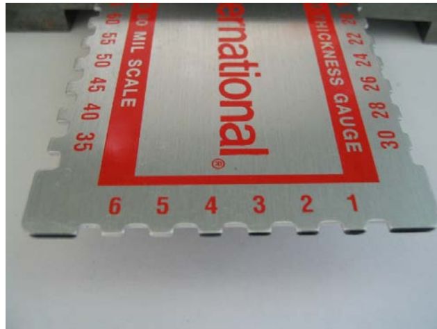
Figure 5. WFT Gauge Showing a Reading of 4-5 Mils.
