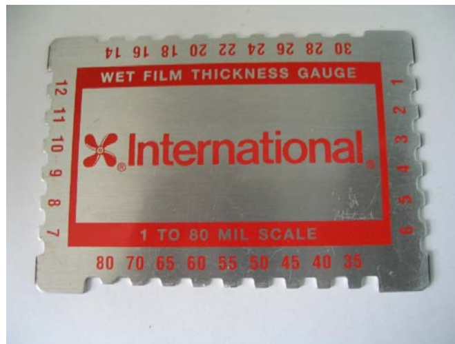
Figure 3. Wet Film Thickness Gauge.
