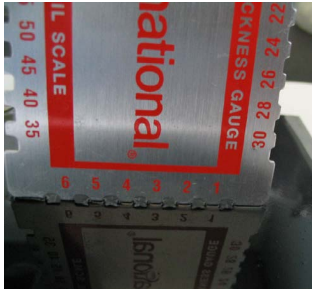
Figure 4. WFT Gauge Positioned in Wet Paint Film.
