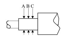
B. FACE RUNOUT, BEARING INNER RING
