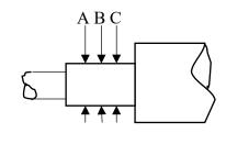
A. SHAFT RADIAL RUNOUT \_\_\_\_\_
