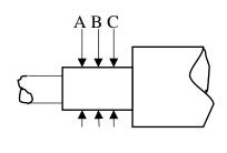
A. SHAFT RADIAL RUNOUT \_\_\_\_\_
