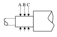
A. SHAFT RADIAL RUNOUT \_\_\_\_\_
