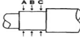
FOR BEARING JOURNAL WIDTH LESS THAN 1 INCH ONLY SIX READINGS ARE REQUIRED.
