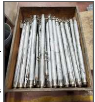
A box of weather deck lifeline stanchions manufactured by NNSY FMB Shop 31A. These removable stanchions are installed topside and provide an extra layer of protection for the crew to reduce the risk of falling overboard. Photo by MR1(SW/AW) Michael Petronio.)
