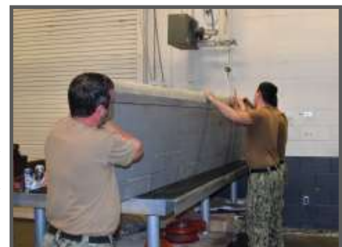
AM2 Steven Bowser, AM2 Mark Rasmussen and AM3 Zane Duty apply leading edge tape in support of a rudder repair. (Photo by LTJG Matthew Starobin.)
