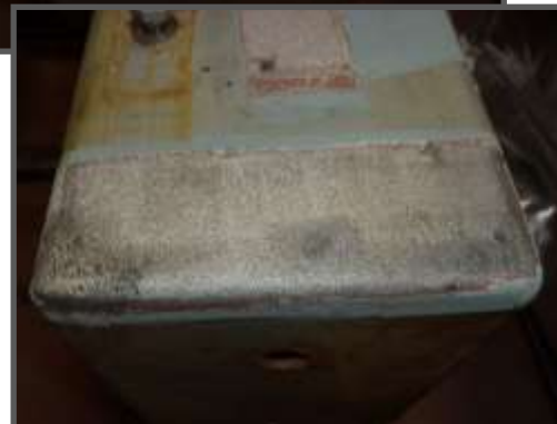
Post after laser ablation; corrosion and paint were stripped from the surface. (Photo by Andy Vasquez.)
