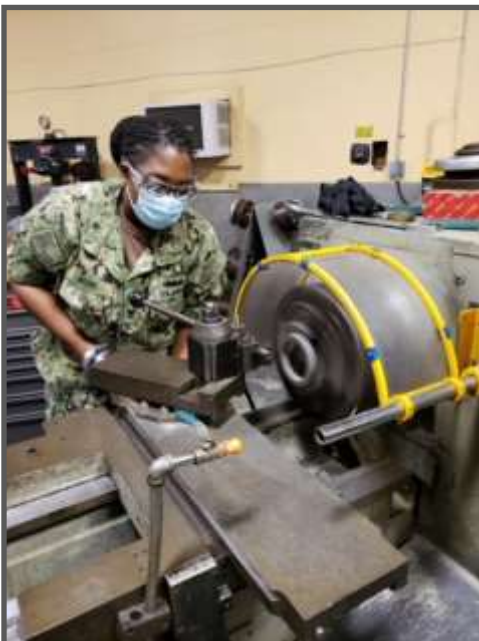
MR2(SW) Taylor Bowie from the NNSY Inside Machine Shop turns a Delrin shim for the stern plane hydraulic cylinder on the USS John Warner (SSN 785). Engine lathes are capable of machining various materials including metal, plastic, and wood. Delrin is a trademarked acetal homopolymer material from DuPont and is known for its high-load mechanical applications such as gears, safety restraints, door systems, conveyor belts, healthcare delivery devices, and other demanding products and parts. (Photo by MR2(SW) Walker Iverson.)
