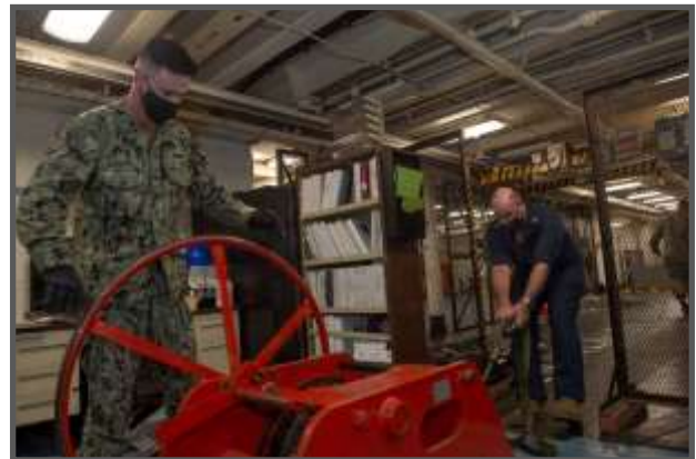
FT2 (SS) Zane Glidewell (left) helps as FT1 (SS) Edward Scaglione prepares a barge winch for weight testing. Scaglione, with the Weapons Department, is currently enrolled in the NAMTS Rigger/Weight Tester JQR and also serves as the Leading Petty Officer of the weapons department's Weight Handling Shop. The shop provides weight testing and handling services and provided 4,851 hours of submarine repair support during 2020. (Photo by MC2 Charlotte Oliver.)
