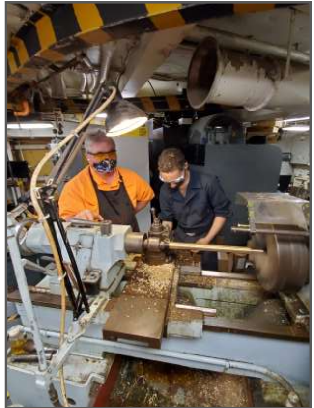
Mr. Rick Smith, NAMTS Inside Machine SME, provides MRFN Kenneth Whitfield training in establishing a reference point during shaft manufacturing. (Photo by Russell Lincoln.)
