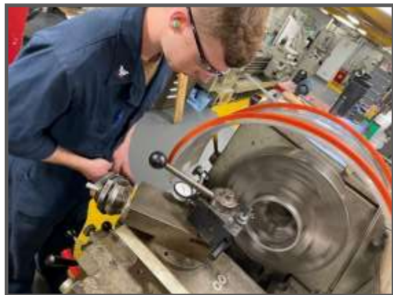
MR3 (SW) Kyle Young putting finishing touches on a pump wearing ring. (Photo by MRC Jesper Sison.)
