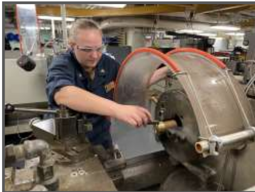
MR2 Stephanie Heppard dresses out threads on a fire-main adapter piece. (Photo by MRC Jesper Sison.)
