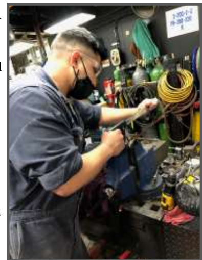
DC2 Victor Cano, Jr., saws the edge of the handle being machined to the appropriate length.
