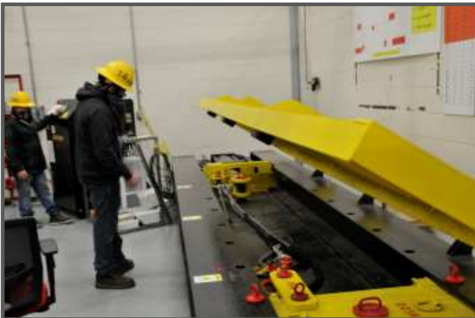
Mr. Bryan F. Mazzitelli (left) and Mr. Nathaniel A. Shrote (right) are testing a pair of RHIB hoisting slings on the 225K Horizontal Proof Test Machine which is computer based, hydraulically operated, and commonly referred to as the pull test machine. (Photo by MR2 (SW) Kevin Lucas.)
