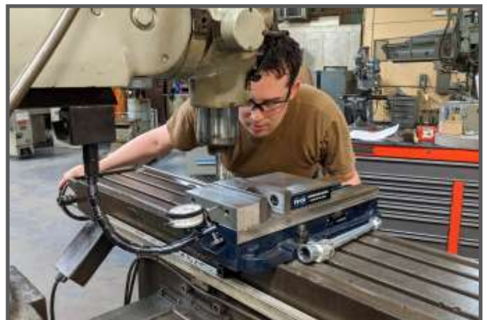
Using a vertical mill in the Inside Machine shop at MARMC, MR2(SW) Marshall Darnell from NNSY manufactures an alignment rod for the USS Washington (SSN-787) out of K-Monel, a non-ferrous alloy containing mainly nickel, copper, and aluminum. K-Monel metal is corrosion resistant, capable of being hardened, and non-magnetic. (Photo by MR1 (AW) Daniel Mendes.)
