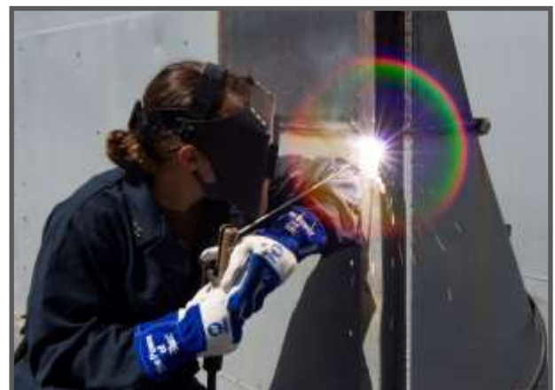
HT2 Pamela Hensley is a member of the Repair Department Hull Repair Division (R-1) and is currently enrolled in the Shipfitter JQR. She is seen here exercising her welding skills in repairing a damaged portion of a bulkhead onboard a floating barge where layout and fabrication were required. With over 100 Hull Maintenance Technicians onboard, R-1 Division provides a myriad of services in submarine repair. It is also a perfect setting for Hull Technicians to earn their NAMTS NEC in Shipfitting and Pipefitting. R-1 currently has 46 Sailors enrolled in NAMTS. (Photo by MC2 Charlotte Oliver.)
