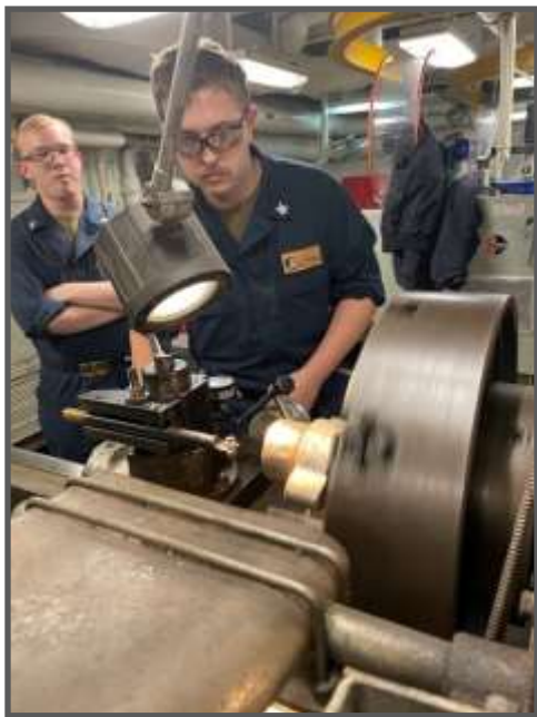
(L-R) MR2 Jared McGregor and MR3 Gabriel Cooper conduct a left-hand threading process. (Photo by MRC Jesper Sison.)
