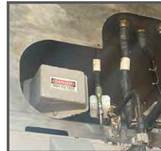
Left: Severe corrosion on an electrical junction box on the main deck affecting the ship's lifesaving system. Note that the bottom of the box cover had heavy corrosion, which could have been affecting the structural integrity of the high voltage box. Right: The same electrical junction box after it was cleaned then treated with Sailor Putty and Sailor Paste; this is a temporary remedy to prevent further corrosion until the unit can be repaired or replaced.
