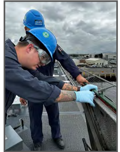
DCFN Noah Steadman (front) and DC3 Devin Rivers conduct an inspection of the gasket on a Quick acting water tight hatch on board an Independence variant LCS.
