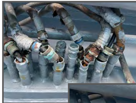
Left: Stuffing tubes and conduit aboard USS Iwo Jima (LHD 7) showing severe degradation due to corrosion. The image below shows the same area after the application of Sailor Putty. (Photos by Darrohn Bickford.)
