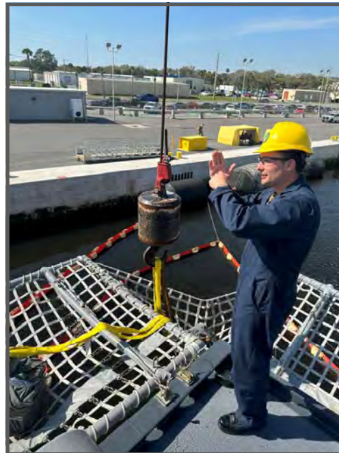
SERMC's BM2 (SW) Brice Smith is aboard USS Marinette (LCS 25) as he sends a signal to the crane operator weight testing flight deck nets. (Photo by BM2 (SW) Jazzment Shanks.)
