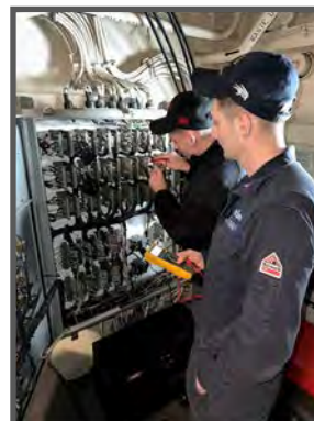
EM2 Dmytro Tsyganovskyi and EM3 Kaleb Stryd are taking readings and checking connections for the solenoids on the ship's stern gate. (Photo by Rizalito Antonio.)
