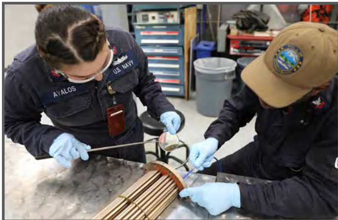
Using a heat exchanger training aide, MM2 (SW) Christopher Louis, demonstrates how to clean a heat exchanger using hand tools to MM2 (SW) Valerie Avalos. (Photo by MM2 (SW) John Rabanes.)
