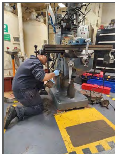
MR3 Robert Figueroa is preparing to install a lubricator holding unit for the Bridgeboard Milling Machine after conducting an after lubricating filter inspection aboard USS Harpers Ferry (LSD 49).
