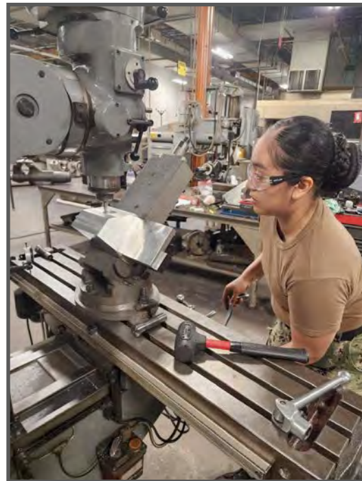
MR2(SW/AW) Mayra Zepedaalvarez uses a Bridgeport Vertical Milling Machine to cut a shape aluminum stock to design specifications. Once completed, this part will be sent to USS Washington (SSN 787) for installation. (Photo by MR1(SW) Taylor Bowie.)
