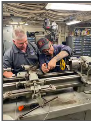
NAMTS Inside Machine mentor Rick Smith (left) provides over-the-shoulder mentorship to MR1 (SW) Thomas Evans, who is installing a valve hand wheel. (Photo by Darrell Monroe.)
