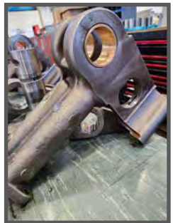
Above: Rocker assembly coated with CPC 500 after one week.
