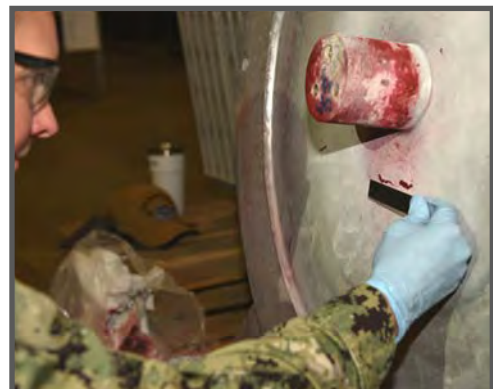
Below: Hull Technician 1st Class Petty Officer Jennifer Schleuning measures cracks that are normally invisible to the naked eye on an upper platform for a ship's brow while conducting non-destructive testing. Schleuning was selected as OPNAV Shore Sailor of the Year for 2023. (Photos by Scott Curtis, SERMC PAO.)
