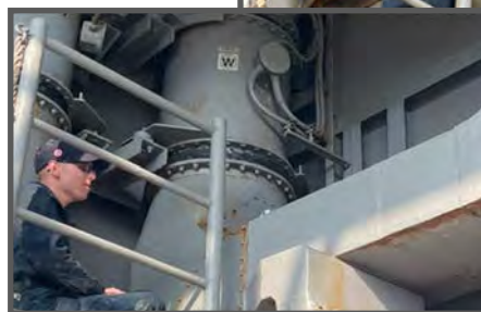
Before (above) and after (left) corrosion mitigation using Sailor Putty and Sailor Paste.
