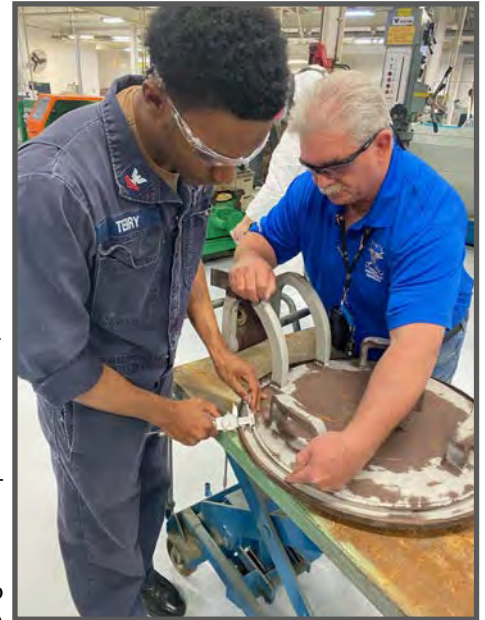
MR2(SW) Nathan Terry measures the water tight scuttle seal area prior to manufacturing a new retaining ring as Rick Smith, Afloat NAMTS Inside Machine mentor provides guidance. (Photo by MR1(SW) Zachery Eisenhower.)
