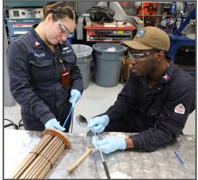
Using a heat exchanger training aide, MM2 (SW) Christopher Louis, demonstrates how to clean a heat exchanger using hand tools to MM2 (SW) Valerie Avalos. (Photo by MM2 (SW) John Rabanes.)
