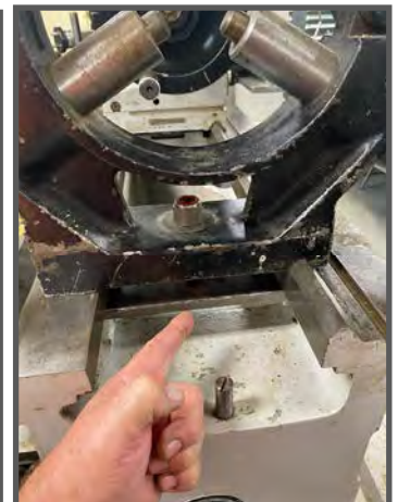
Left: NAMTS Inside Machinist mentor points out to HTFN Malkowski that the Lathe steady rest mounting bracket was missing.
