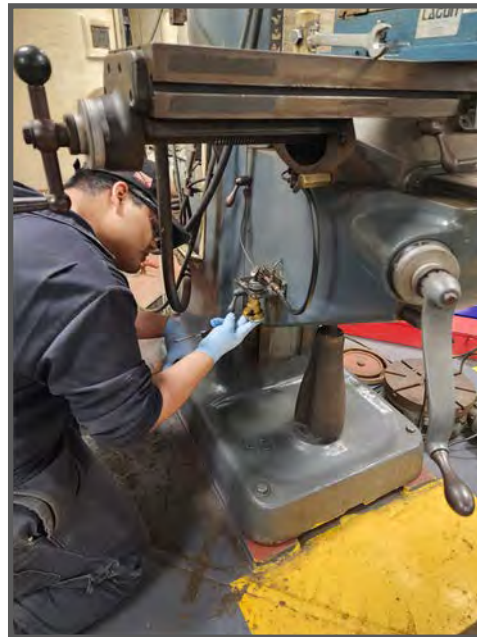
MR3 Robert Figueroa inspecting the lubricating filter before installing the lubricator holding unit for the Bridgeboard Milling Machine.
