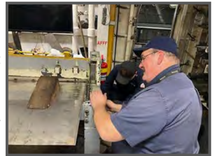
NAMTS Structural mentor Alton Kinchen (right) provides over-the-shoulder mentorship to HT3 Shandon Tsosie with shear guides adjustments. (Photo by Steven Constantino.)
