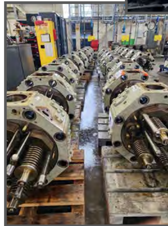
Cylinder heads coated with CPC 500.
