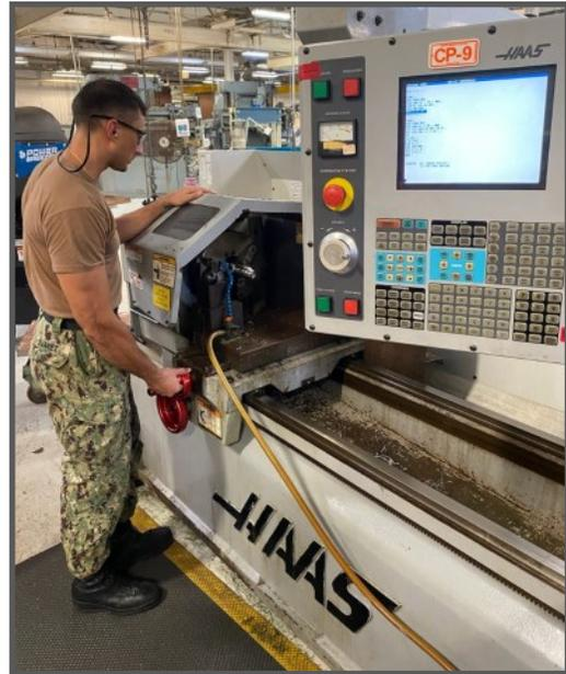
NAMTS Sailor, MR2(SW) John Suarez, positions the CNC Lathe cutting tool into home position before activation of the CNC machining process of a deck plug at Southeast Regional Maintenance Center (SERMC) Code 941, Inside Machine Shop. (Photo by Rick Smith.)
