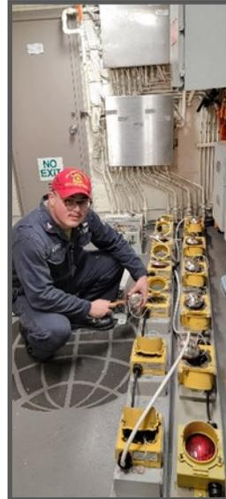
While EM2 Oscar Alfaro is conducting repairs on the vertical dropline lights, NAMTS Electrical SME Rizalito Antonio took the opportunity to provide over-the-shoulder mentorship guidance for principles found in the NAMTS Outside Electrical Repair Technician JQR. Vertical drop line lights serve as an extension of the deck lineup lights and provides the pilot with continuous lineup during night approach. (Photo by Rizalito "Tony" Antonio.)
