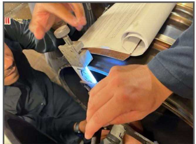
*GSM1 Daye is conducting a ROV on #3 Gas Turbine Generator aboard USS Daniel Inouye (DDG 118).*
