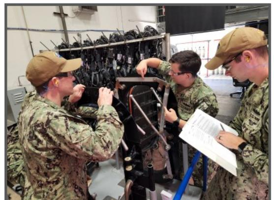
DC2(SW/AW) Britton Raven (center) is giving NAMTS training to DC2(SW) Robert Yarborough (left) and DC2(SW/AW) Austin Williamson (right) by identifying the parts of the conrod assembly on a Quick Acting Watertight Door (QAWTD).
