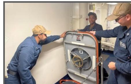
L-R: MR3 Jordan Point being assisted by Divisional Damage Control Petty Officers EN3 Courtney Davis and FC2(SW) Steven in safely placing Watertight Hatch in a safe maintenance position in order to properly conduct a gasket channel inspection and gasket replacement. (Photo by Ramir Pulido.)
