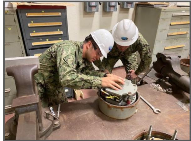
MM2(SW) Michael Bailey and MM2(SW) James Lokey inspect a pad-eye electric motor brake for proper air gap clearance. The air gap needs to be close enough to catch once the brake is activated but not too close to cause dragging. This procedure is one of the more common jobs in the MARMC Outside Machine Shop. (Photo taken by MM2(SW) Jonathan Lepley.)
