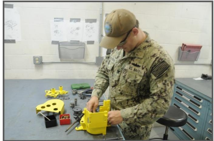
FC3 (SW) Christopher Bowdenwright installing a cartridge guide on an ammunition loader.
