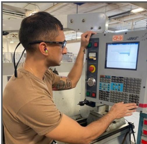
MR2(SW) John Suarez programs thread diameter requirements into a CNC Lathe for manufacturing a deck bolt at Southeast Regional Maintenance Center, Inside Machine Shop Code 941. (Photo by Rick Smith.)
