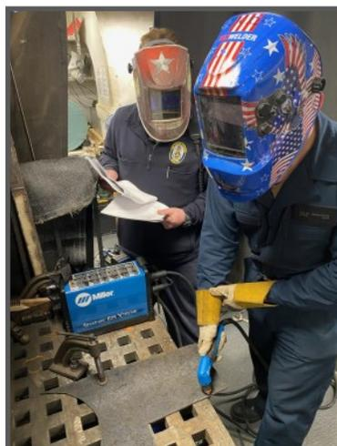
HTFN Colin Chasten prepares to use a plasma cutter to cut out a part from a sheet of carbon steel aboard USS Jason Dunham (DDG 109). (Photo by MMC(SW) Gordon Reichert.)
