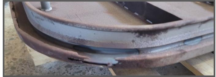
A corroded watertight door is kept in the shop as a sample of severe degradation. (Photo by Doug Scholl.)
