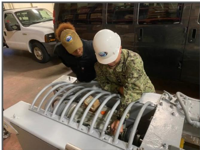
MM2(SW) Kareema Webb and MM2(SW) Michael Bailey make adjustments to the flexible coupling on a sliding pad-eye off USS Stout (DDG-55). The flexible couple is used to absorb a slight misalignment with the main electrical motor and the ball screw. (Photo by MM2(SW) Jonathan Lepley.)
