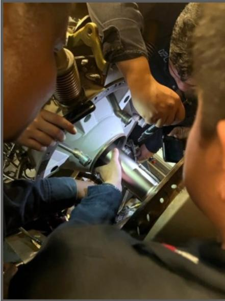
Gas Turbine Repair Shop 38MH, is mating the combustor to diffuser on #2 Gas Turbine Generator aboard USS Daniel Inouye (DDG 118). (Photo by Philip Bowler.)
