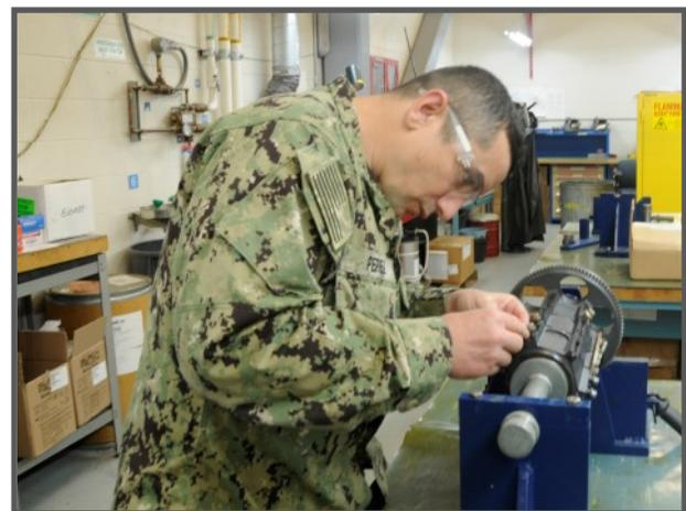
FC1 (SW/AW) Alexander Perez lockwiring remover track spacers on a CIWS gun rotor.
