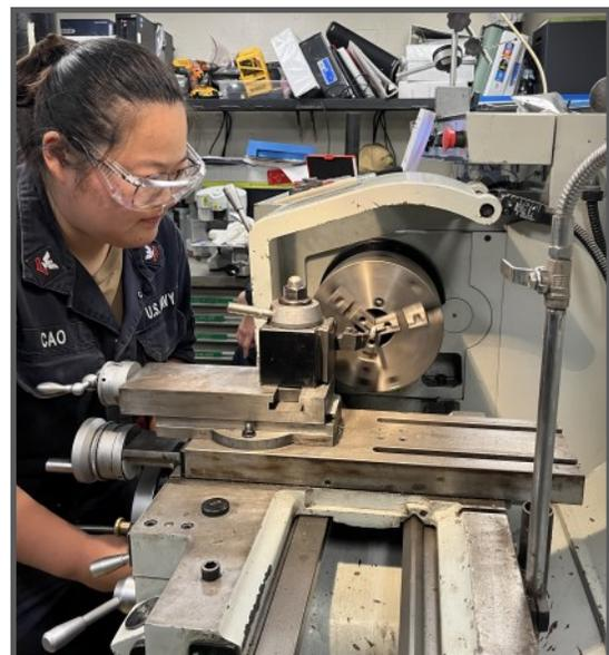
MR2 Yingli Cao uses the lathe aboard USS John Finn (DDG 113) to manufacture a shear pin to fix a lathe.
