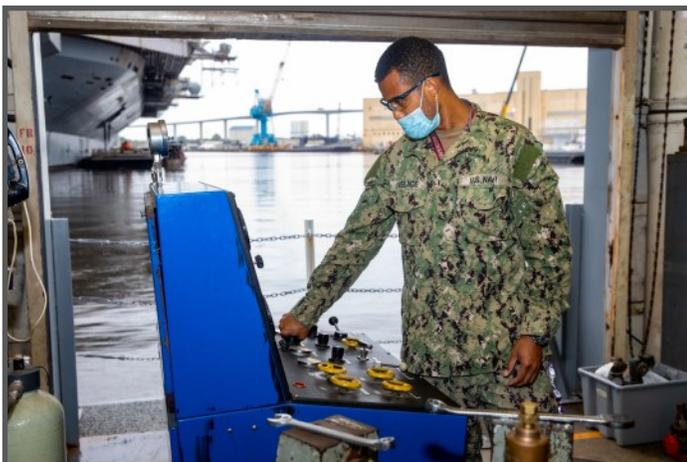
A Sailor on the NNSY Valve Barge operates a test stand to hydro test relief valves. (Photo by NNSY Photographer, Mrs. Shelby West.)
