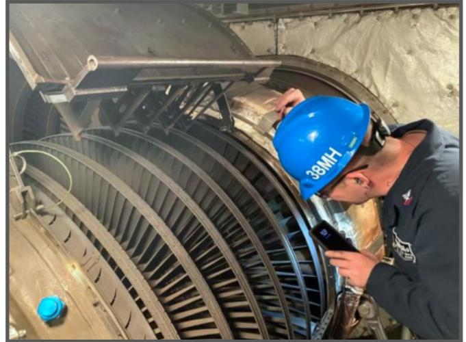
*GSM2 Schillinger is conducting a Gas Turbine Bulletin 12 inspection on a Turbine.*
