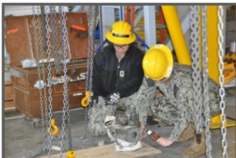
BM2 Eileen Pasion, with the assistance of BM2 Cheyenne Moscoco, verifies the lashings on this valve are properly torqued prior to lifting. (Photo by Sandy Hinz.)
