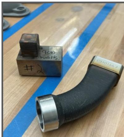
The item on the left is a test print from a Haas UMC 750 that was printed at 900 watts of laser power from solid 304 stainless steel weld wire. The part on the right was previously created by welding three parts together; it is now printed as a single component. (Photo by NAMTS Public Affairs.)
