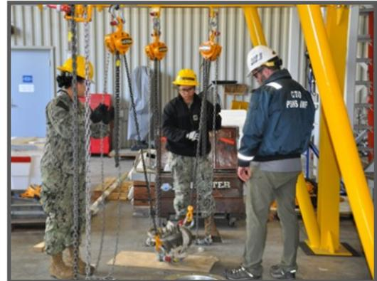
Mr. Brody Denis observes as BM2 Eileen Pasion and BM2 Cheyenne Moscoco carefully lift a valve during a Rigger / Weight Tester practical examination. (Photo by Sandy Hinz.)
