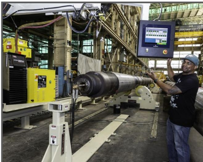
Welding Supervisor Donovan Harris shows how to use the control panel for the newly acquired Computer Numerical Controlled (CNC) Submerged Arc Welder (SAW) at Norfolk Naval Shipyard on July 12, 2021. (Photo by Aldo Anderson.)
