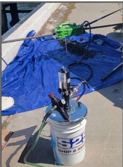
The VIPER system removes debris while it injects new lubricant all in one motion, eliminating Sailors exposure to HAZMAT. (Photo by Andy "Rusty" Vasquez.)
