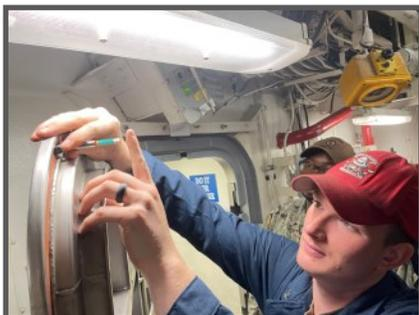
DC3(SW) Nathan Harris conducting a permanent set / groove measurement in the MAFO-Holtkamp door gasket with DC1(SW) Jonson Fraiss observing. (Photo by Ramir Pulido.)
