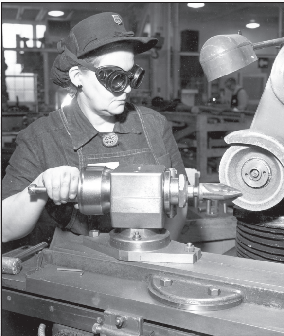
1945—An employee works with a countersink sharpening fixture, which was developed and built by Shop 06.
