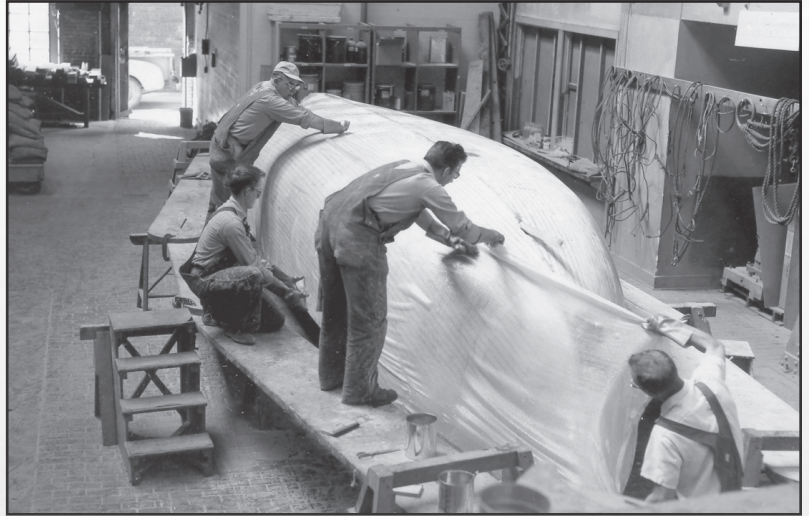
1957—Production workers apply woven roving to the outside skin of a small boat.
