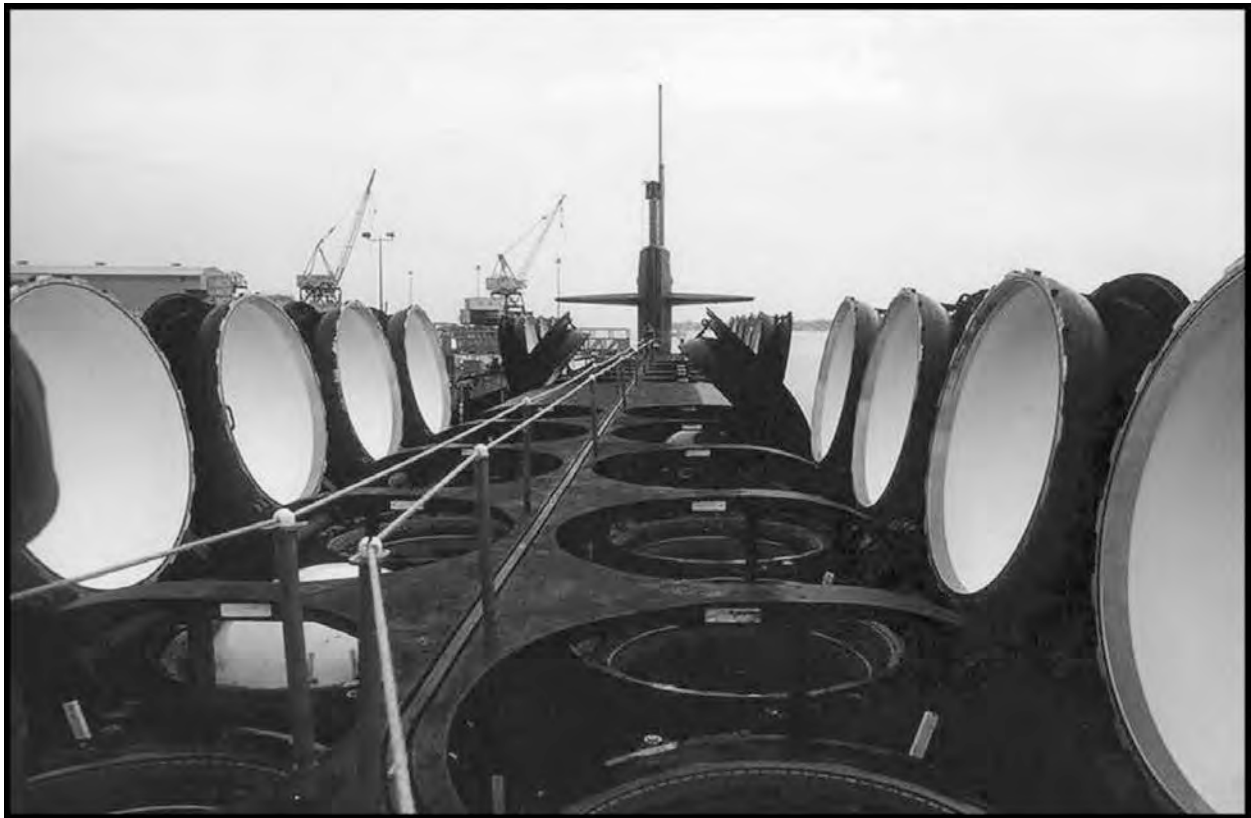
USS OHIO (SSGN 726) with her missile doors open. OHIO was the first of four SSBNs to complete conversion to SSGN.
