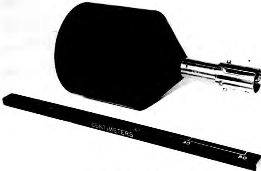
Fig. F56-1 - Type F56 transducer.
