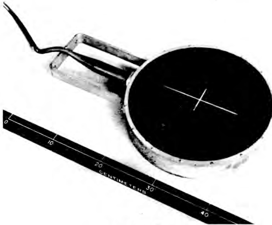
Fig. F27-1 - Type F27 transducer
