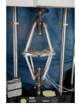
fabrics, composites, elastomers, metals, biological tissues and other complex materials, reducing the need for expensive full scale testing. The fixtures provide multi-axial and shear mechanical data for analysis in one apparatus and can be used in conjunction with finite element models for designing new materials and minimizing the number of prototypes required. Fixtures are available for licensing or for use in collaborative design of new materials.
