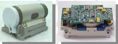
OLD NEW FA-18 GYRO COTS INSERTION & RELIABILITY IMPROVEMENT
