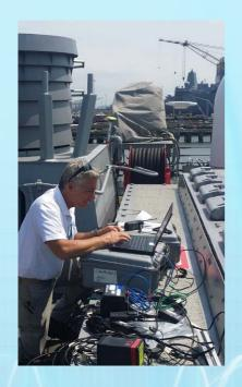
The ship's plans and technical data are used during the dockside phase to determine the location of each sensor onboard relative to the FORACS reference point.
