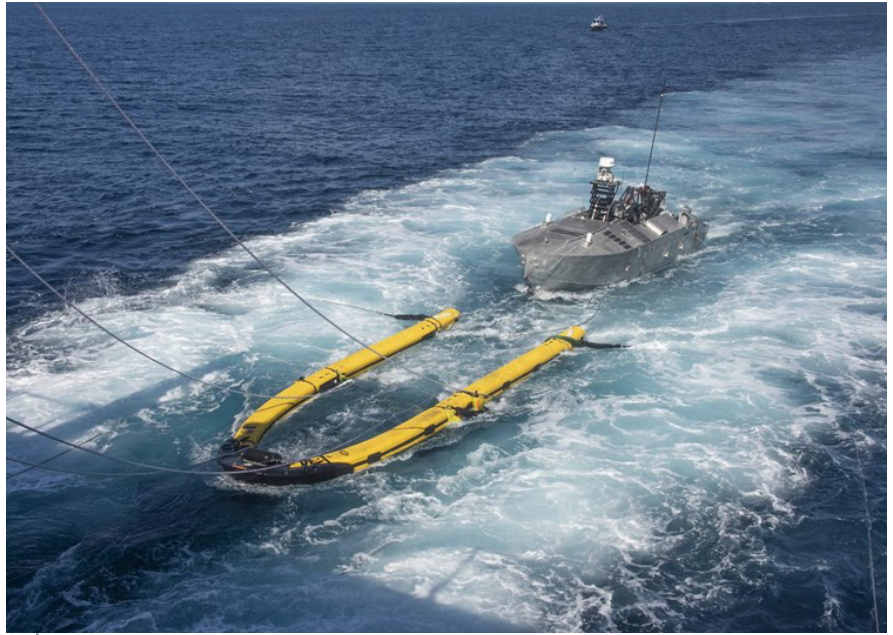
The Mine Countermeasures Unmanned Surface Vehicle (MCM USV) in Minehunt configuration performs launch and recovery operations during Initial Operational Test and Evaluation (IOT&E), Aug. 2022. (U.S. Navy photo by Ronnie Newsome)
