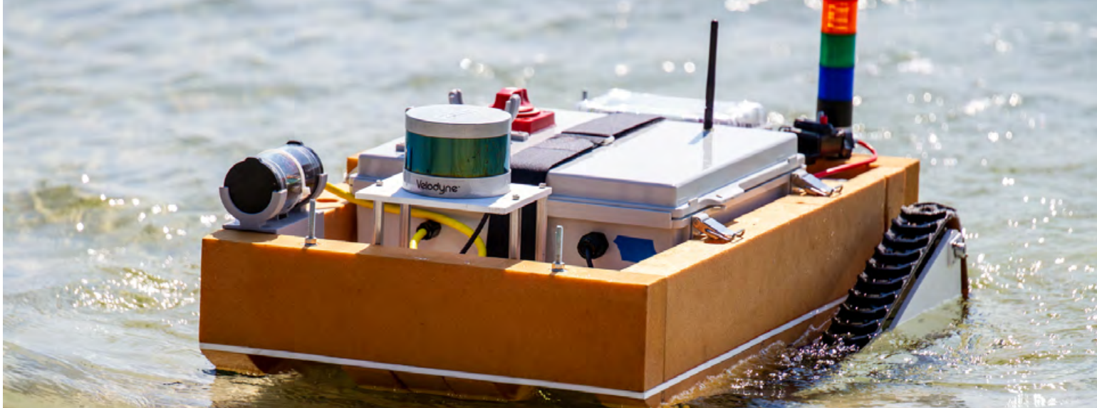
X Department's – "The aXolotls" – amphibious vehicle transitions from water to land during preliminary trials of the Technical Director's Cup. They chose to build an amphibious vehicle capable of autonomous navigation both on land and at sea, quickly transitioning between the two, according to X Department Team Captain Melanie MacBain.
