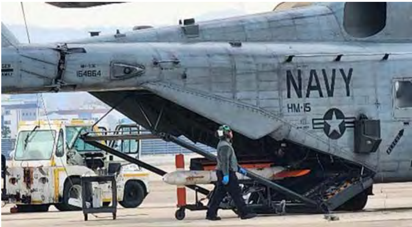
AN/AQS-24 being loaded aboard MH-53 helicopter.
