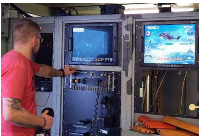
Technician monitoring AQS-24 performance during maintenance event.
