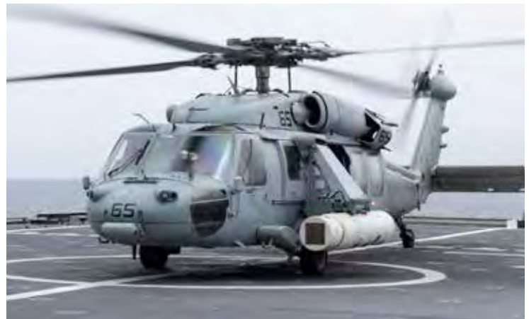
ALMDS installed on the MH-60S Knighthawk helicopter
