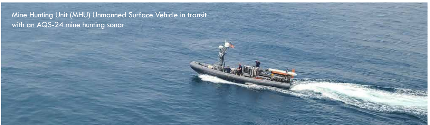
AQS-24 launched from a Mine Hunting Unit (MHU) Unmanned Surface Vehicle.
