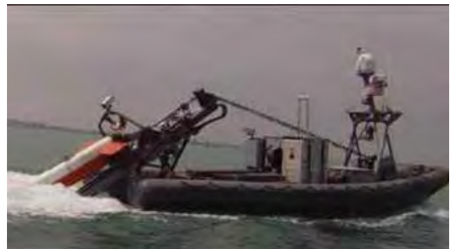
AQS-24 launched from a Mine Hunting Unit (MHU) Unmanned Surface Vehicle.
