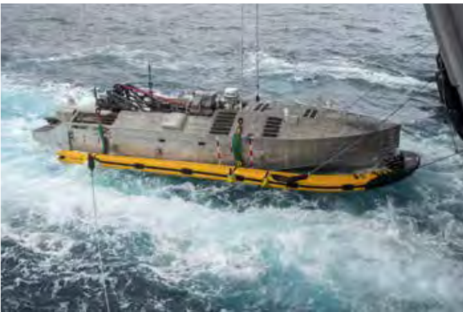
MCM USV being launched from the littoral combat ship
