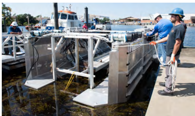
Pharos receives final preparation before launching into the water to test its ballasted and de-ballasted loaded configurations.
