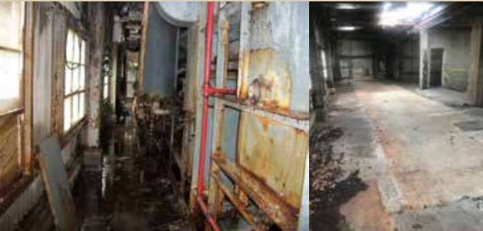
Before and after explosives decontamination high bulk density nitroguanidine manufacturing equipment (tobacco dryer at building 498).
