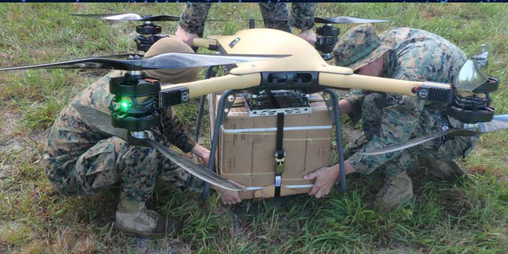
In May, DAT members conducted their final operational demonstration of the Unmanned Logistics System – Air Joint Capability Technology Demonstration program at Fort A.P. Hill, Virginia. U.S. Marines and Soldiers planned and executed cargo deliveries while flying the TRV-150 unmanned aerial vehicle with autonomy packages. Flown to remote landing zones, delivered materials include ammunition crates, meals ready to eat (MREs) and large containers of water. A key mission objective of the program is to deliver cargo weighing up to a ton within five hours.
