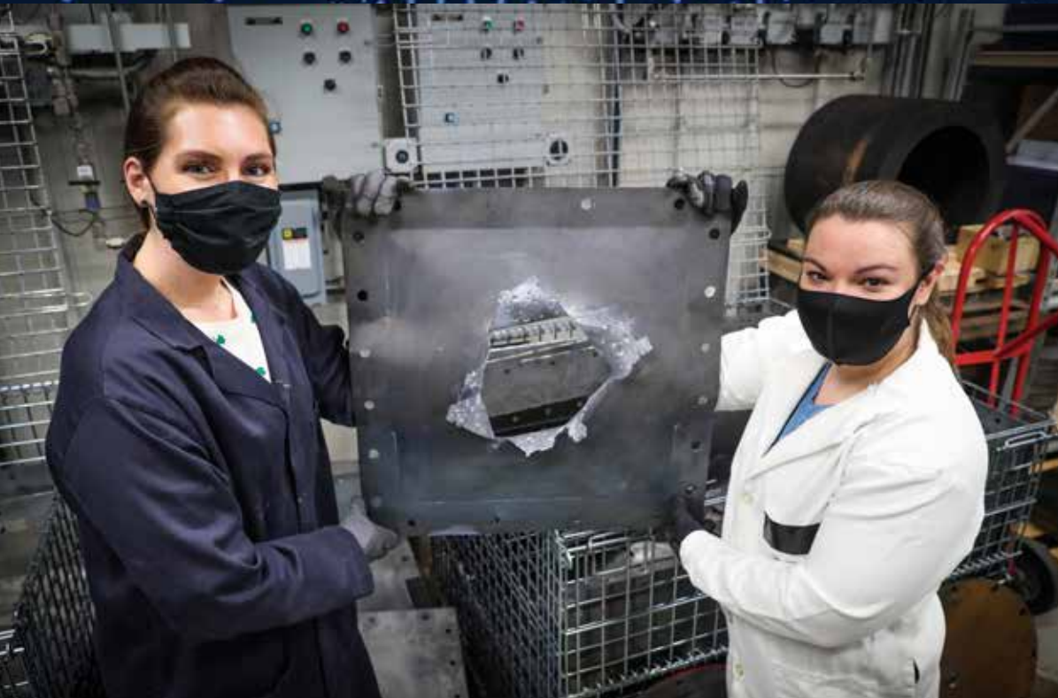
RDT&E Department Materials Science Branch scientists Dr. Alexandra Reinert and Dr. Anne Haslam designed and implemented a new testing apparatus for characterizing high-speed reactive material impact and penetration events in March. Pictured: Reinert (left) and Haslam (right) display an example witness plate from current vented chamber calorimetry experiments geared towards screening a subset of novel and preexisting materials.
