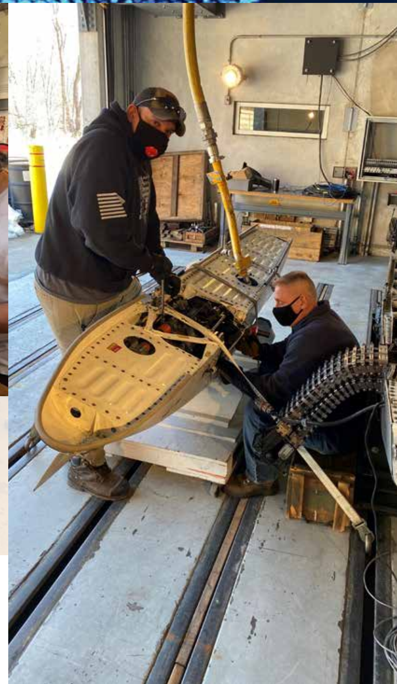
NSWC IHD Picatinny Detachment NAVAIR Medium Caliber Gun ISEA team members David Barlieb and Tommy Singer performed testing on GAU-12 projectile sensors at Range 647. They were tasked with testing excess turned in and repaired sensors for functionality. The units that pass will be returned to the fleet for use as spares in the AV-8B Harrier aircraft. Ten of the 22 projectile sensors passed testing, thus providing spares for fielded GAU-12 gun systems, increasing its maintainability and ability to continue supporting the mission.
