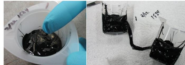
Liner is applied to the inside surface of the tubes, and then the propellant is cast onto the liner, so the liner bonds to the metal, and the propellant bonds to the liner.
