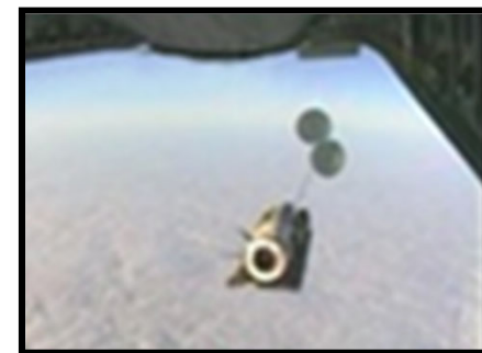
Ballistic missile target being loaded and launched from a C-17 aircraft
