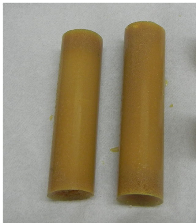
Cured Neat HTPA shows signs of crystallization
