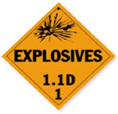
Identifies munitions' damage potential during transportation and storage
