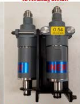
Figure 11, 0.17 and two 0.54 sec delay installation, forward Ejection Seat (MKUS16LA/ MKUS16LB)
