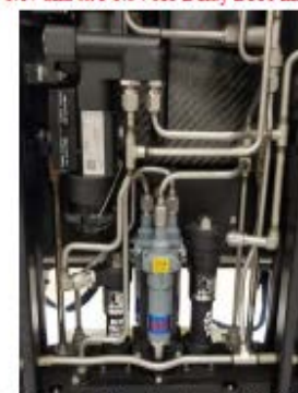
Figure 12, 0.17 and two 0.54 sec delay installation, forward Ejection Seat (MKUS16LA/ MKUS16LB)
