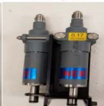
Figure 4, 0.17 sec delay installation (2), rear Ejection Seat (MKUS16LA/ MKUS16LB)
