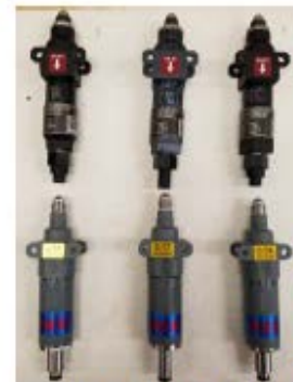
Figure 11, 0.17 and two 0.54 sec delay installation, forward Ejection Seat (MKUS16LA/ MKUS16LB)
