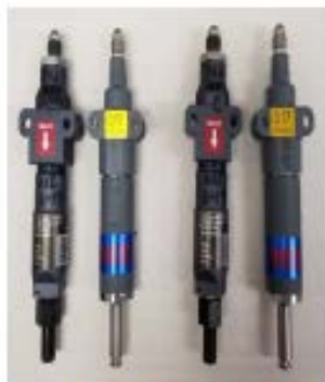
Figure 4, 0.17 sec delay installation (2), rear Ejection Seat (MKUS16LA/ MKUS16LB)
