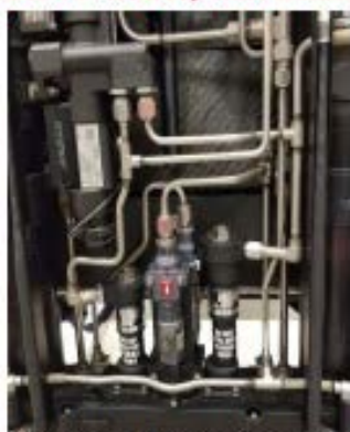
Figure 5, 0.17 sec delay installation (2), rear Ejection Seat (MKUS16LA/ MKUS16LB)
