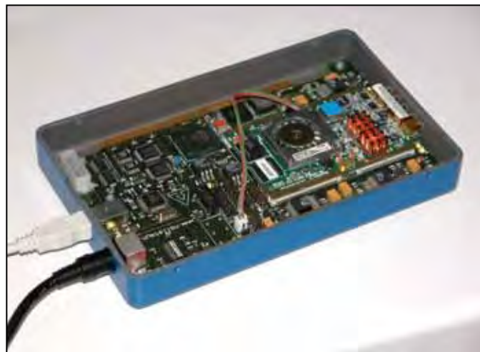
Figure 4. Hardware Platform Used for the FMCW Radar Signal Processor
