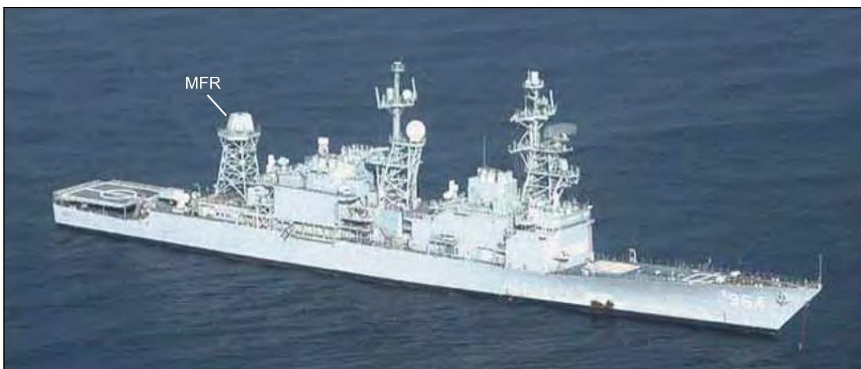
Figure 1. AN/SPY-3 Multifunction Radar (MFR) Installed on SDTS
