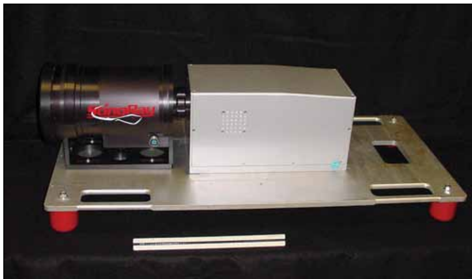
Figure 1. Titanium Camera with the Stingray Optics on the Mounting Plate Part of Its Environmental Enclosure
