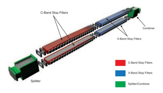
Figure 4. Diagram of the AN/SPS-48 Transmit Waveguide Filter
