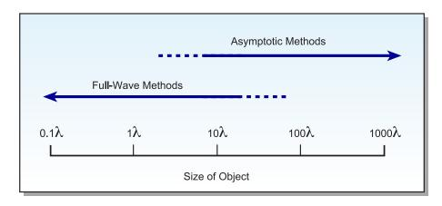
Figure 3. Range of Applicability of Methods Used in CEM
