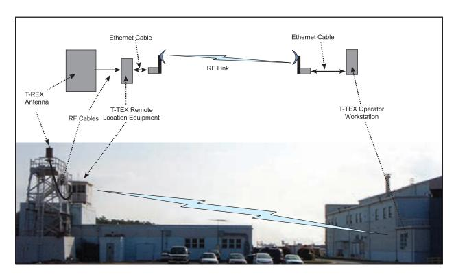
Figure 6. NSWC Dahlgren Evaluation Installation Prior to PMRF Deployment
