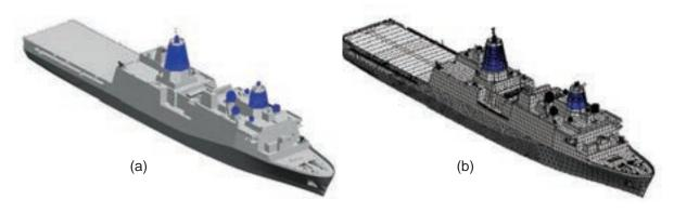
Figure 5. (a) Model of the LPD 17; (b) Mesh of the LPD 17
