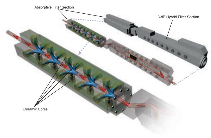
Figure 3. AN/SPS-67 Waveguide Gasless Filter
