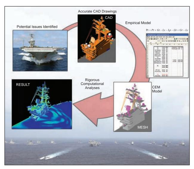
Figure 4. CEM Modeling and Simulation Process
