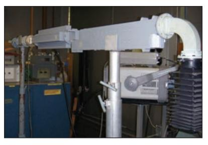
Figure 4. Waveguide Filter Connected to 1 Megawatt Magstand for Power Test
