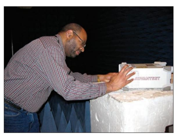
**Figure 3.** An NSWC Dahlgren employee adjusts a spectrum analyzer—a tool used to perform a typical spectrum certification measurement.
