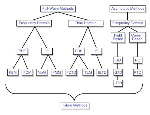
Figure 2. Various Computational Methods Used in Computational Electromagnetics
