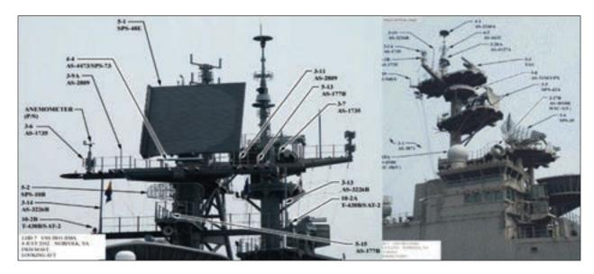
**Figure 4.** Numerous antennas competing for limited space and coverage result in a complex electromagnetic environment (EME), presenting a challenge for effective topside integration and maintaining the topside baseline.
