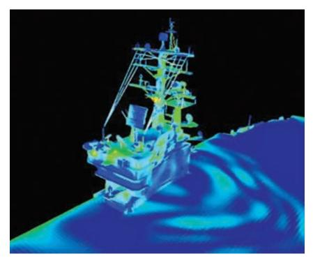
Figure 9. Induced Currents on an Aircraft Carrier Island and Deck
