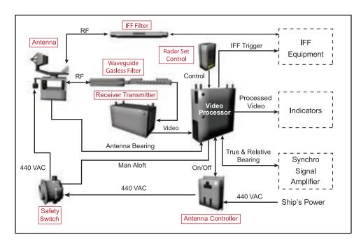
Figure 1. The AN/SPS-67 Radar System
