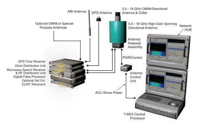
Figure 4. T-REX Remote Site System Components
