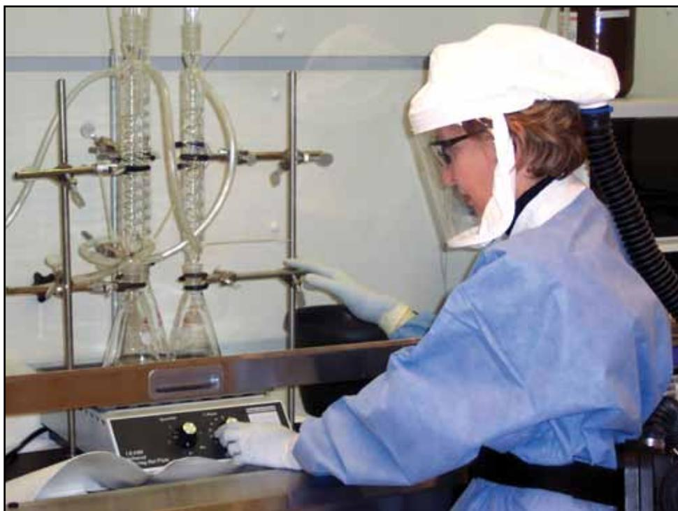
**Figure 3.** Scientist Working in a Toxin Laboratory With a Powered, Air-Purifying Respirator
