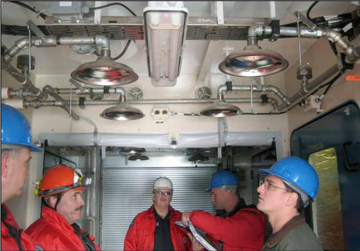
**Figure 2.** Decontamination Station and Shower Aboard the SFD's Fireboat *Leschi*
