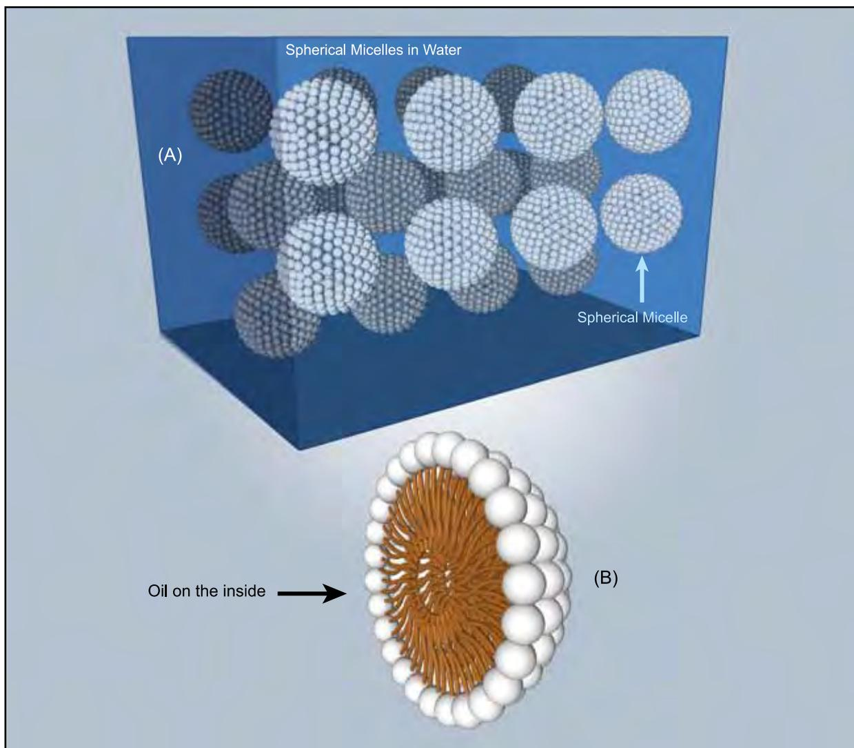
**Figure 4.** (A) Spherical Micelles in Water (B) Cross-Section of a Micelle—Micelles cause oil and water to mix by encapsulating oil droplets and carrying them into the water.
