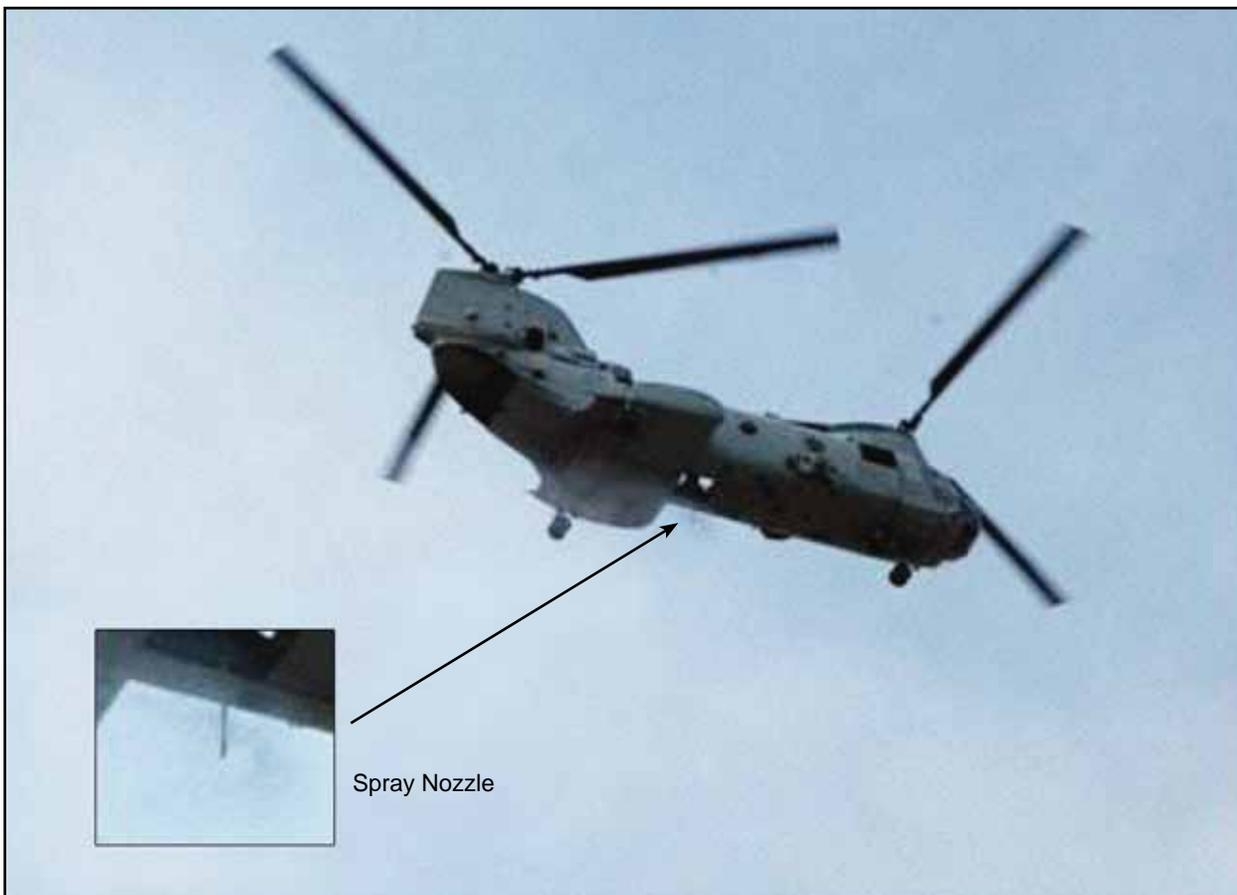
**Figure 3.** Helicopter Spraying Simulated Agent
