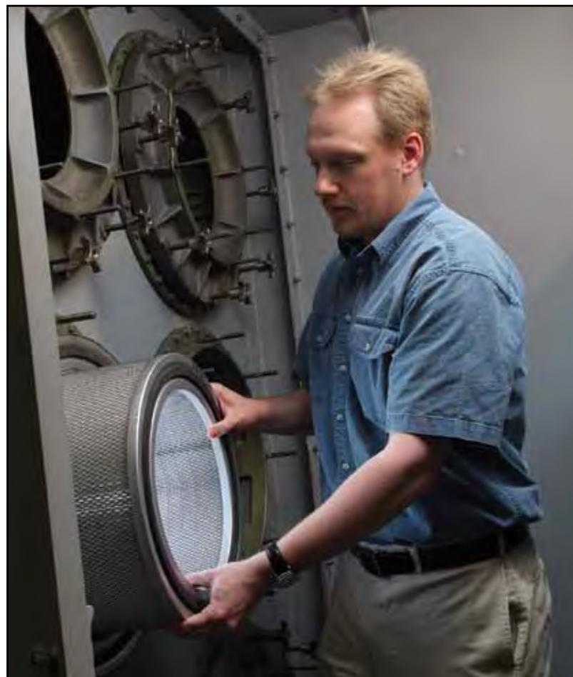
**Figure 1.** An engineer inside the CBR Filtration Evaluation and Support Facility demonstrates a filter change-out procedure.
