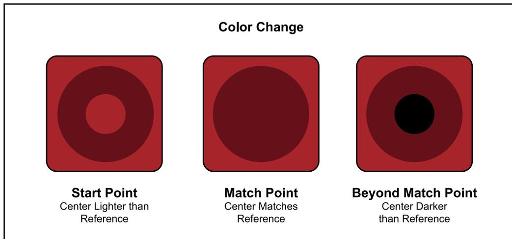
**Figure 3.** Time Temperature Indicator
