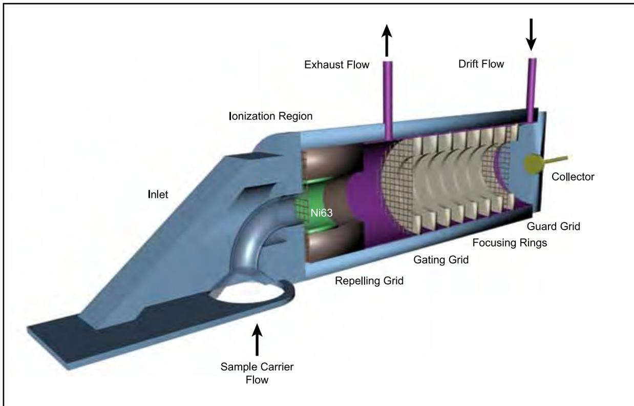
**Figure 3.** Example of an IMS Cell
