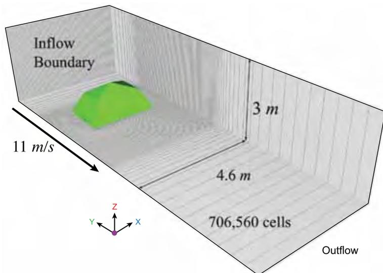
Figure 3. Grid and Domain for the Two-Man Tent in a Wind Tunnel
