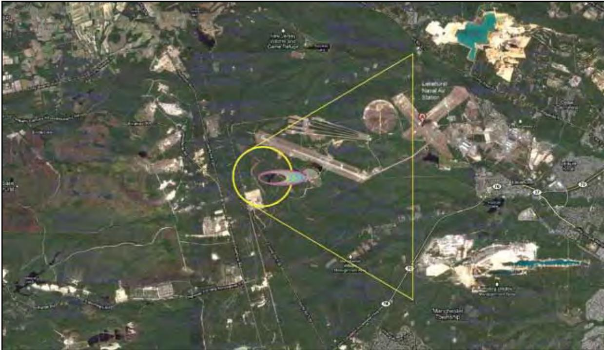
**Figure 2.** COP with JWARN Plot (Yellow) and JEM Hazard Prediction (Blue)—The COP displays the areas that need to be contained or avoided with a NATO ATP-45 triangle of the impacted area.
