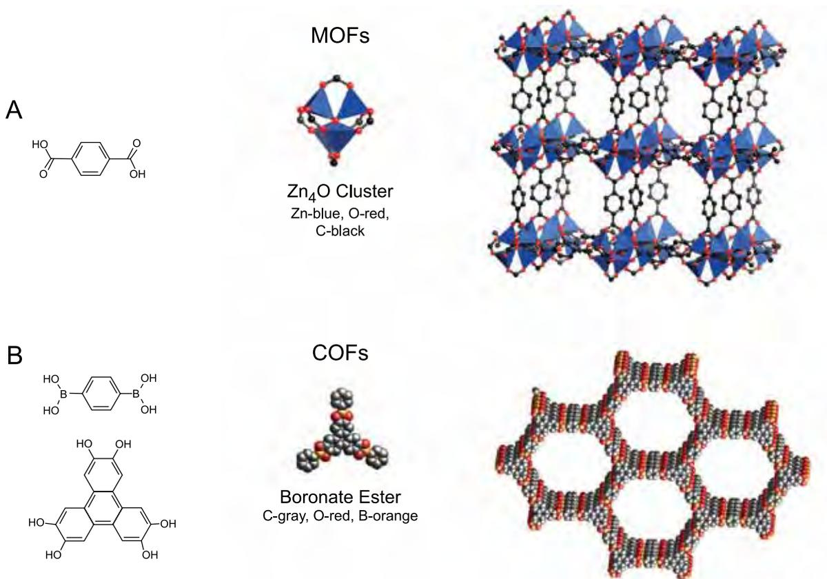
**Figure 1.** Synthesis of MOFs (A) and COFs (B) showing the formation of building units from organic linkers and metal ions and the extended structures formed from these building units.
