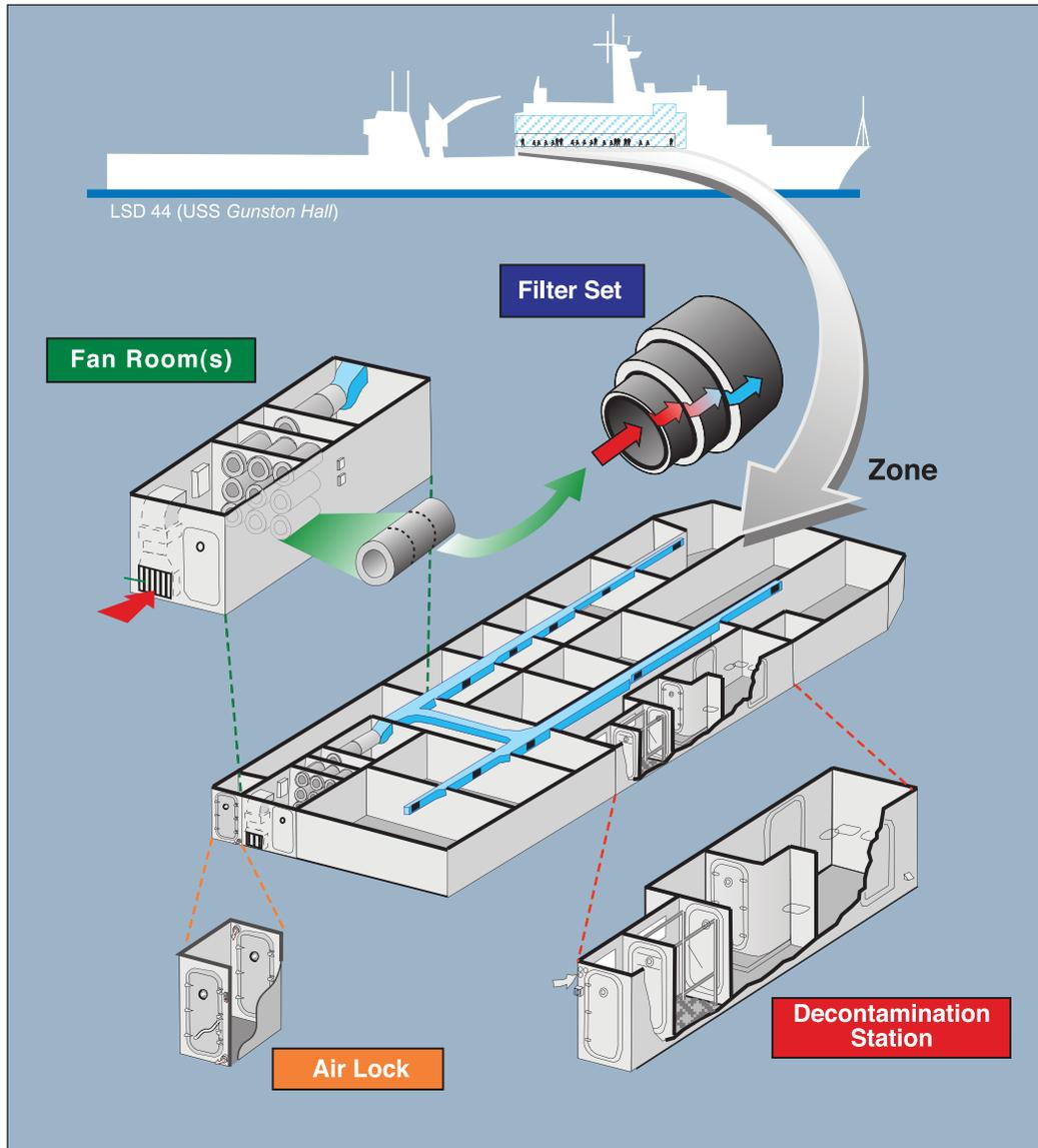
Figure 1. Layout of a Typical Collective Protection System Zone
