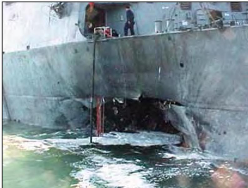
**Figure 2.** Damage to USS *Cole* From a Terrorist Attack: The CPS greatly enhanced rescue and recovery efforts and also limited the extent of damage on the ship.
