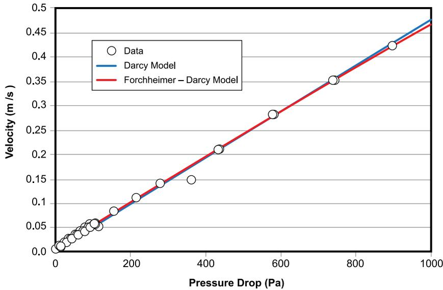
Figure 2. Measured Velocity as a Function of Pressure Drop Across a Triosyn Filter
