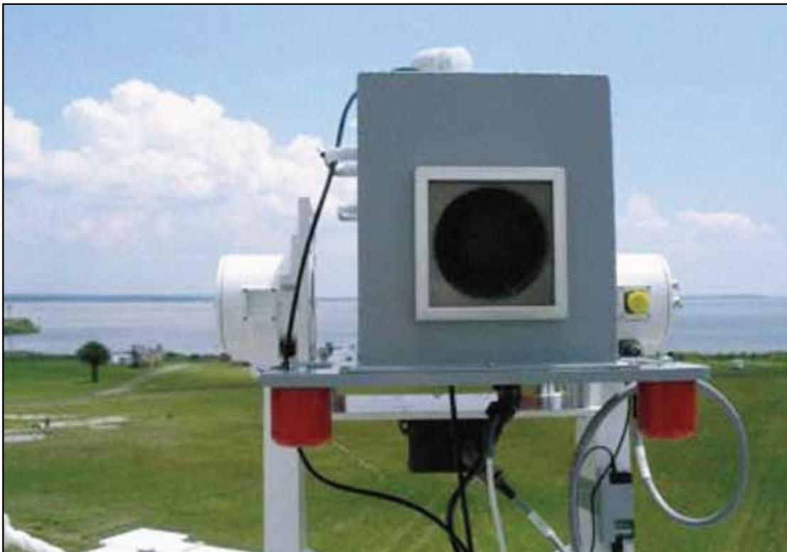
**Figure 2.** View from the CBRD Facility overlooking the Potomac River Test Range (PRTR)—This IR sensor focuses on a very narrow frequency band to detect agents and simulants by their absorption of IR energy at “fingerprint” wavelengths.
