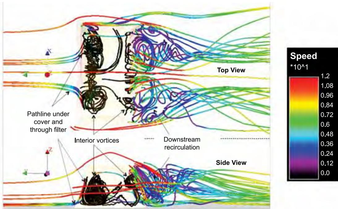
Figure 4. Top- and Side-View Particle Paths Around and Inside Tent
