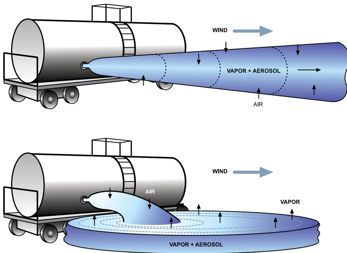
Figure 1. TIC Vapor Plume Formation Versus Pooling at the Release Site
