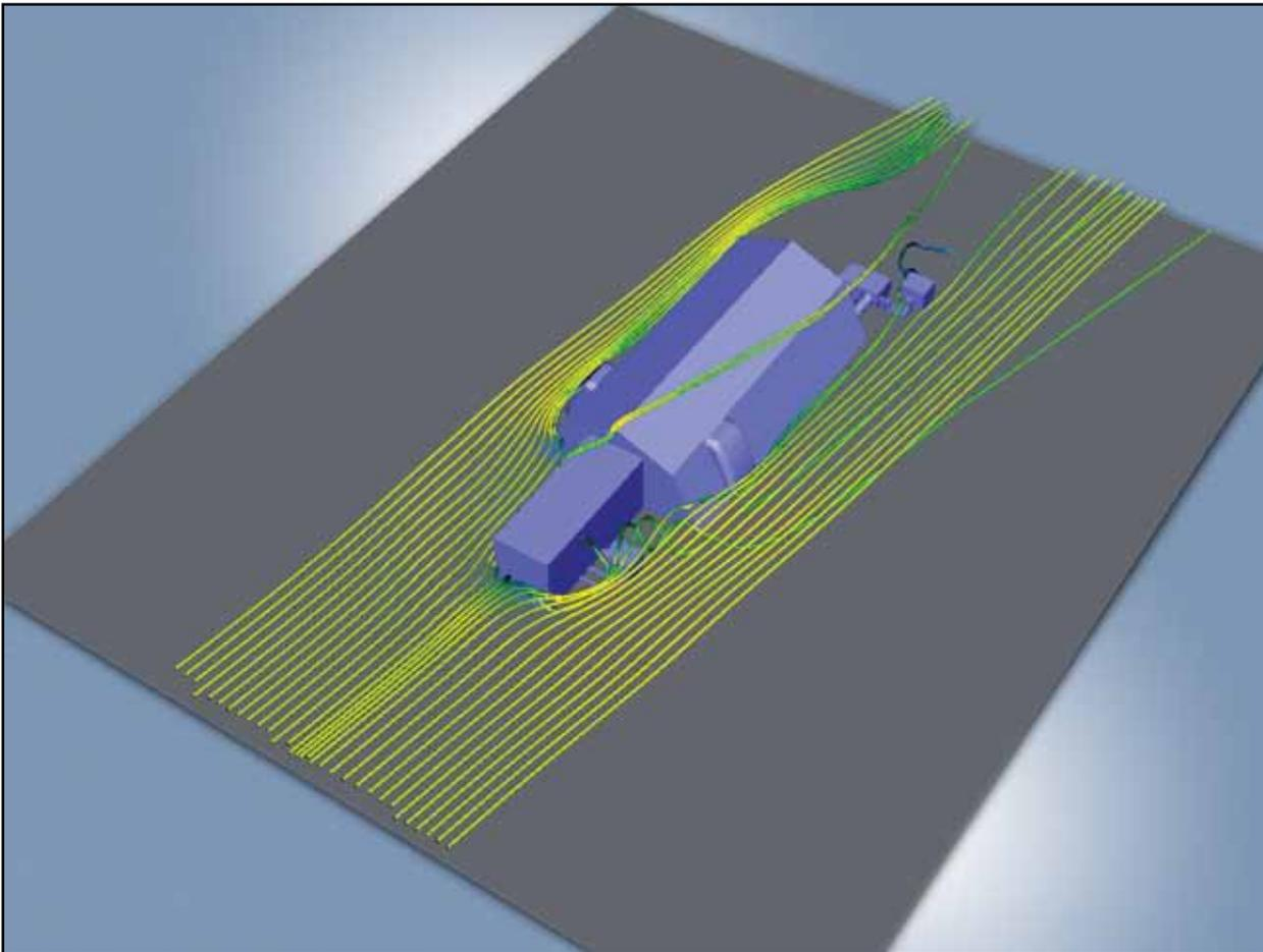
Figure 1. Airflow Over a Shelter
