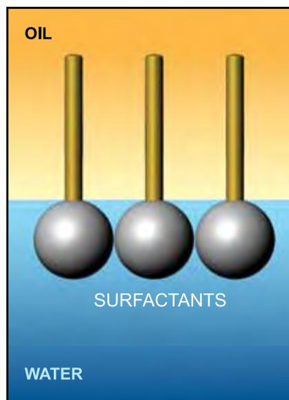
Figure 3. Surfactants reside at the oil and water interface. The hydrophilic group prefers to bond with water, and the lipophilic group prefers to bond with oil.
