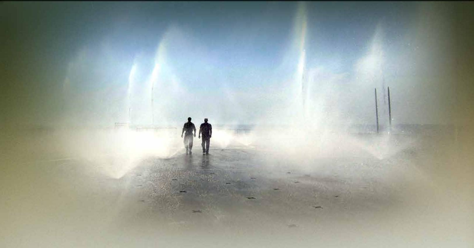
Persian Gulf (May 28, 2005) – Sailors assigned to USS *Ashland* (LSD 48) inspect the sprinklers and valves of the chemical, biological, and radiological (CBR) wash down system on the ship's flight deck. USS *Ashland* is currently conducting Maritime Security Operations in the Northern Persian Gulf.
