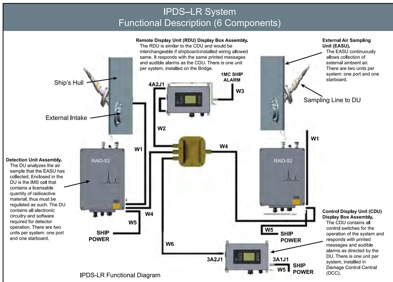
**Figure 5.** IPDS-LR external air sampling units sample exterior air and transfer it to the detector units (DUs) for analysis. Two exterior points are sampled and alarm/status is communicated to two points in the ship: Damage Control Central and the Bridge.
