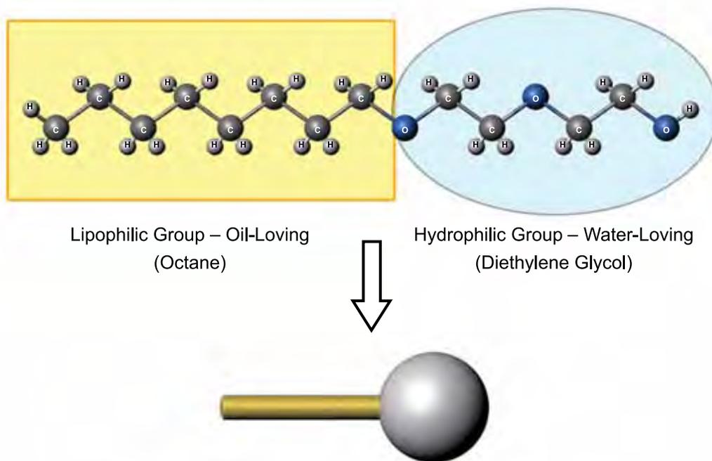
Figure 2. Simple Model of a Surfactant
