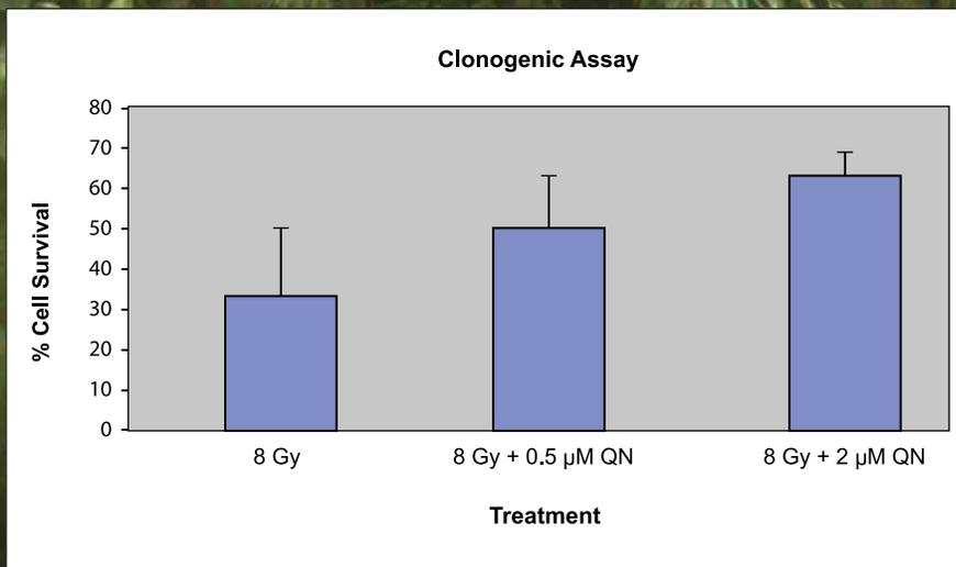
**Figure 3.** After exposure to 8 gray (Gy) of radiation, approximately 35 percent of human skin cells survived. Pretreating these cells with various concentrations of quercetin (QN) dose-dependently increased the amount of cell survival, suggesting that this flavonoid compound may have potential as a protective agent for both the warfighter and civilians.<sup>b</sup>
