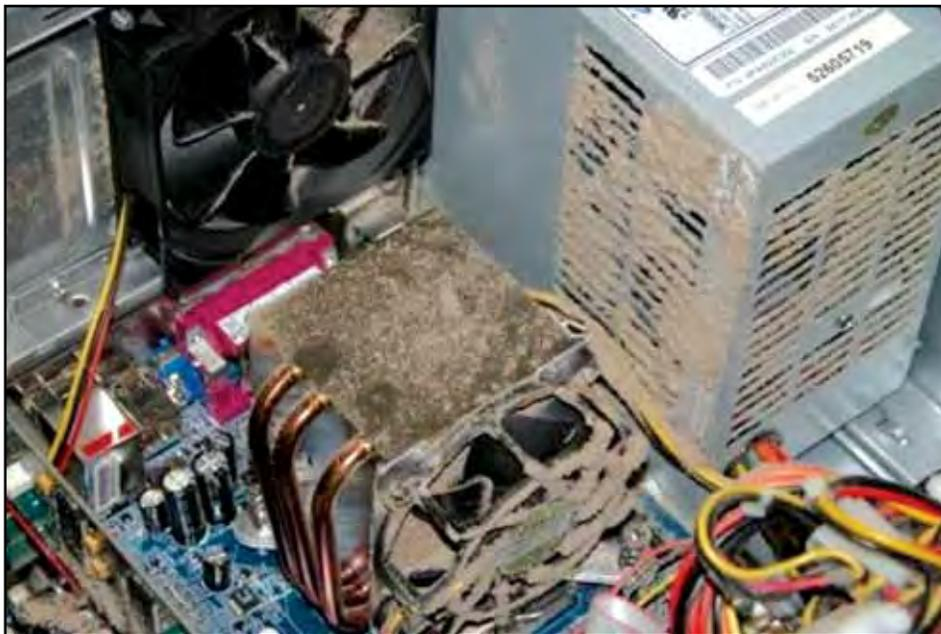
Figure 4. Typical Dust Buildup in an Electronic System
