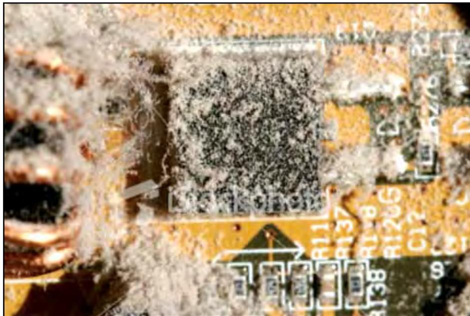
Figure 5. Dust Buildup on a Typical Electronics Board
