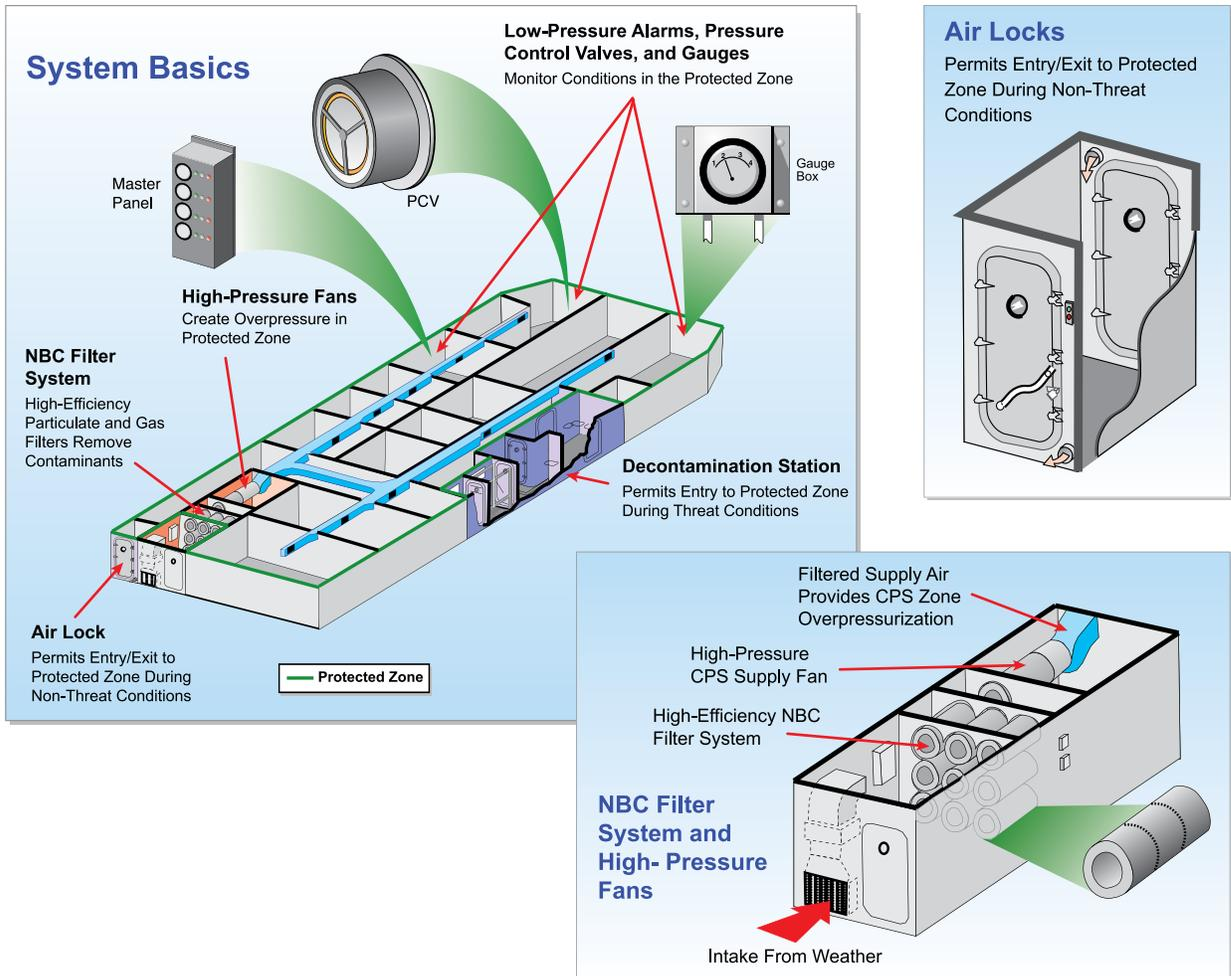
Figure 1. Overview of a Collective Protection System
