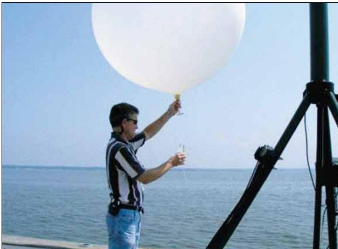
**Figure 3.** A meteorologist releases a weather balloon prior to a test event—Weather data fed into high-resolution models is used for event prediction and for postevent analysis.
