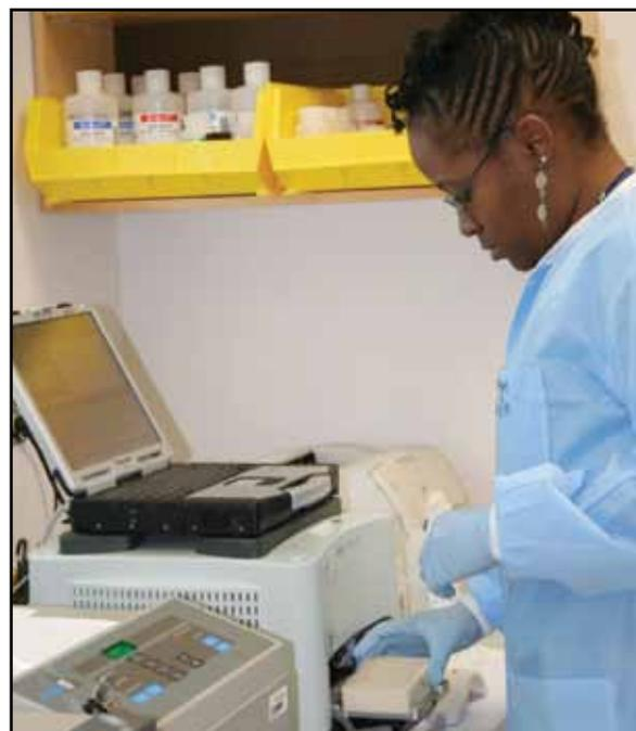
**Figure 1.** Scientist Operating the BioVeris M1M Used for Electrochemiluminescence (ECL) to Detect Bacteria, Viruses, and Toxins/Proteins
