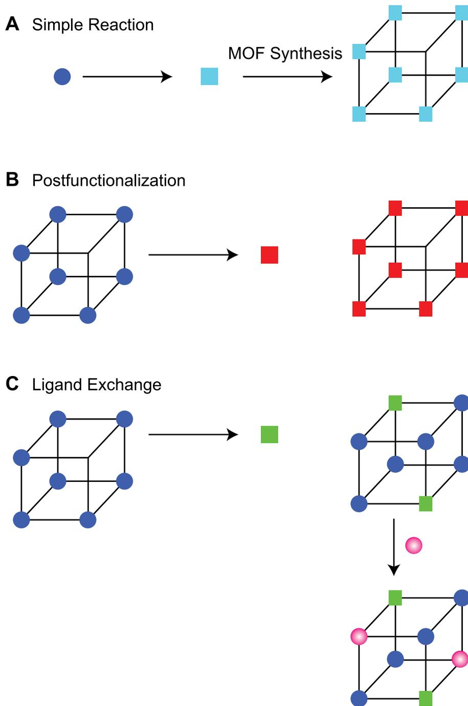
**Figure 3.** Various methods of MOF, COF functionalization: (A) Represents direct transformation of the building block followed by synthesis of the MOF or COF, (B) Postfunctionalization involves modification of the building blocks after synthesis of the extended structure, and (C) Ligand exchange involves sequential exchange of some of the building blocks in the structure after the MOF is synthesized.
