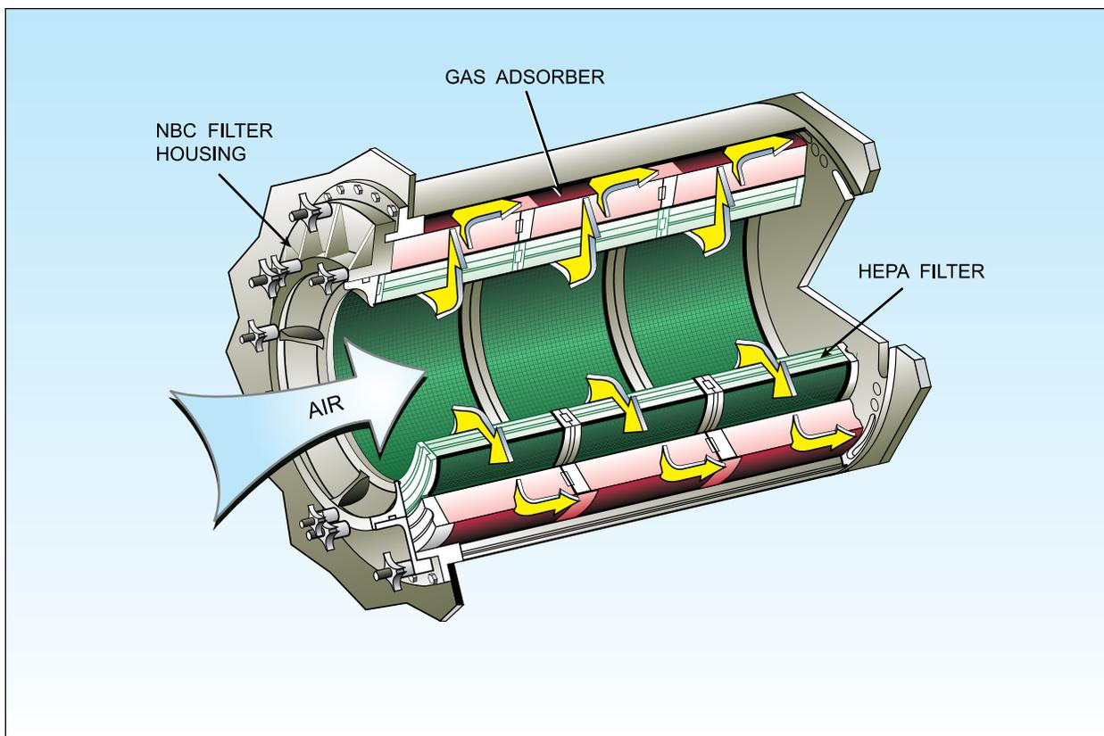
**Figure 1.** M98 Filters Installed in Series
