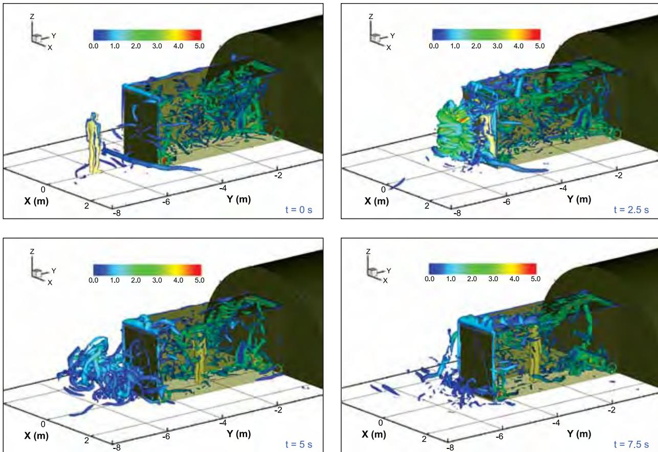
**Figure 2.** Snapshots of Vortex Cores (Colored by Agent Concentration) During a Simulated Entry Into an Air Lock
