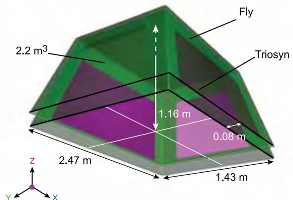
Figure 1. Photograph and ADVEDS Model of the Two-Man Tent Structure
