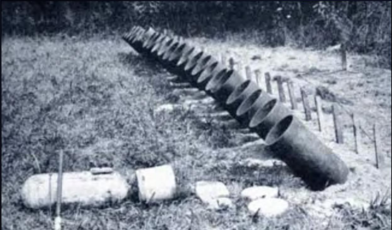
**Figure 1.** A Battery of Dug-In Livens Projectors with One Gas Shell and Its Propellant Charge Shown in the Foreground<sup>4</sup>
