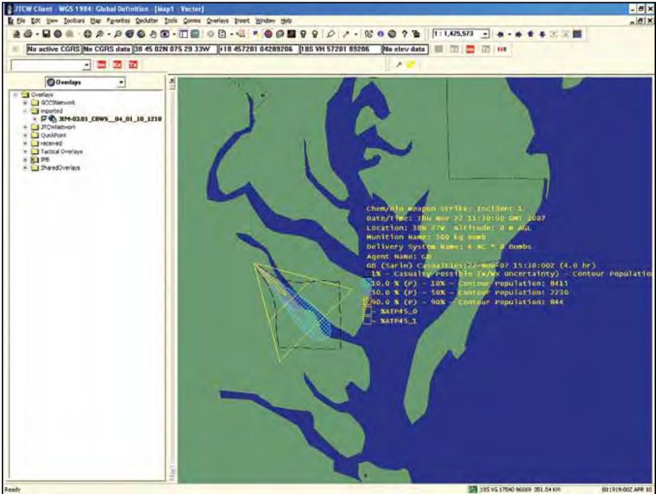
**Figure 2.** Sample JEM hazard prediction from 32 bombs each filled with 500 kg of the nerve agent Sarin. The yellow triangles show the “old” method of estimating the hazard. The dotted black lines show the possible uncertainty in wind direction. The colored contour plots show three different levels of Sarin toxicity predicted by JEM.
