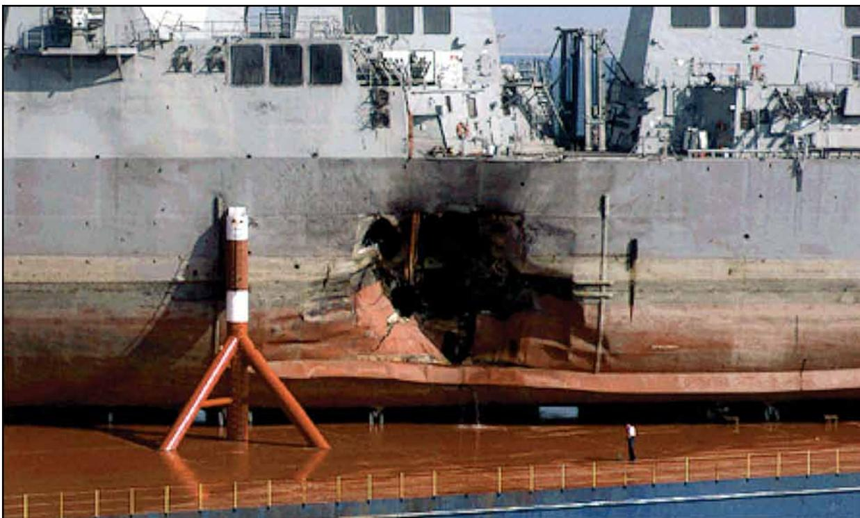
**Figure 1.** Damage Caused by the Terrorist Attack on USS *Cole* (DDG 67) in October 2000
