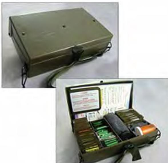
**Figure 2.** M272 Water Testing Kit
