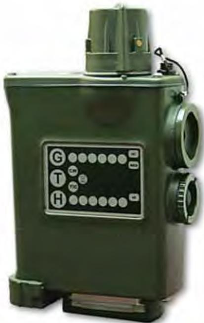
**Figure 4.** Joint Chemical Agent Detector (M4) (JCAD)
