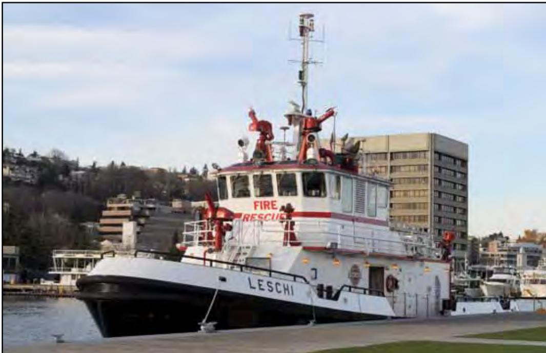
**Figure 3.** The *Leschi*, built in 2007, is a 108-foot fireboat that can shoot 22,000 gallons of water per minute and travel at 14 knots.
