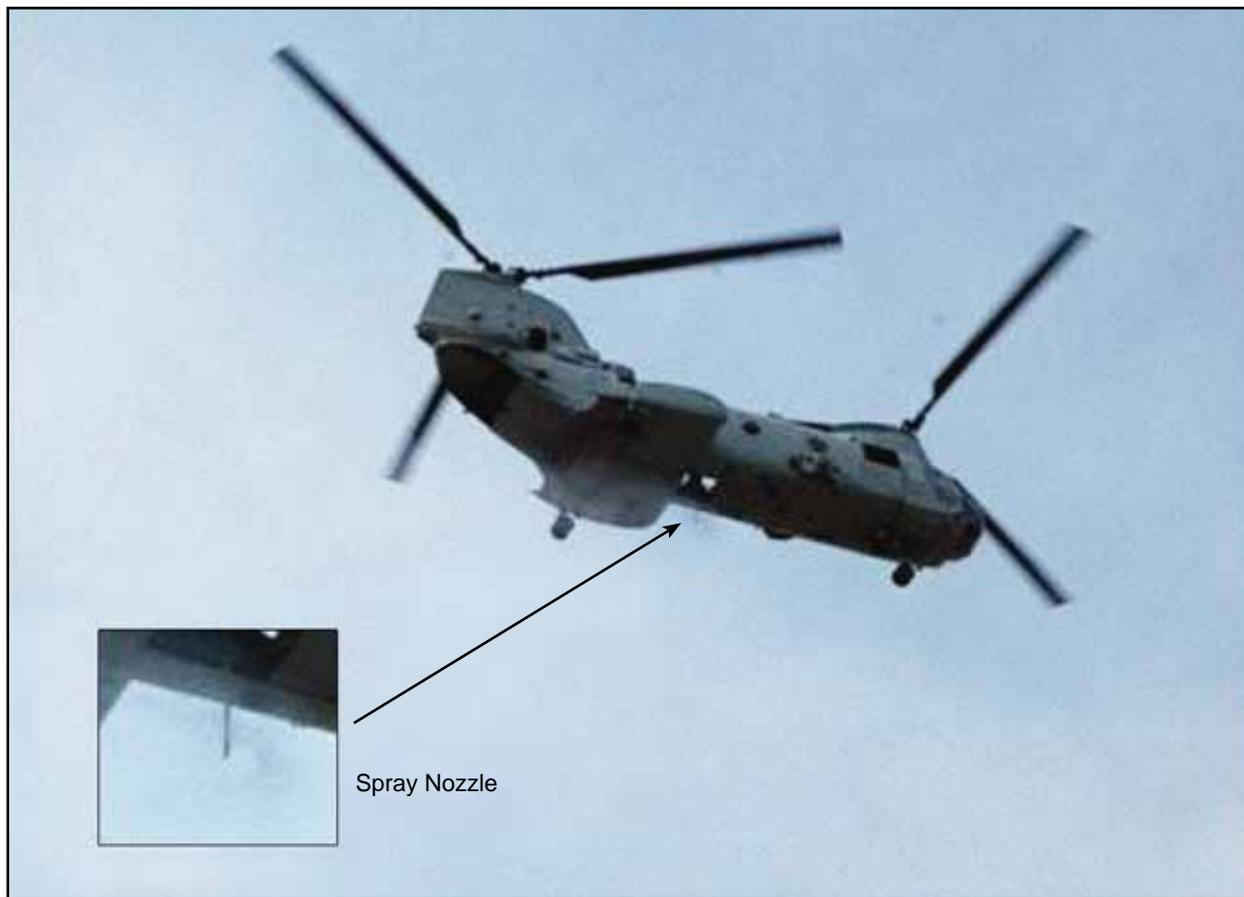
**Figure 3.** Helicopter Spraying Simulated Agent
