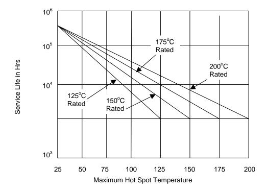
Figure 1. Service Life vs. Hot Spot Temperature
