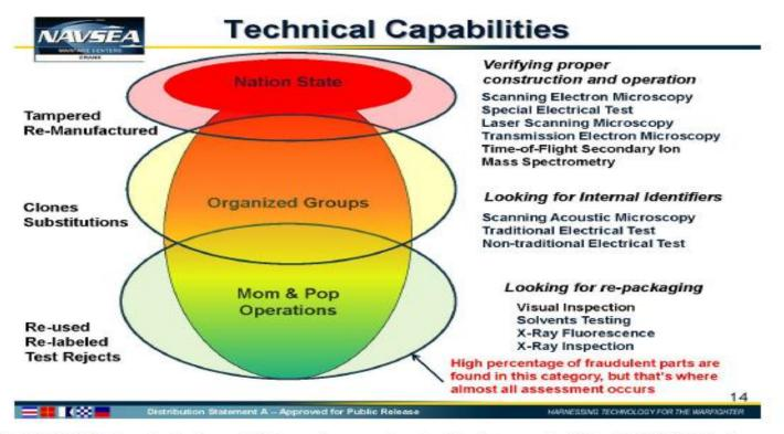
FIGURE 2-2 Technological capabilities and approaches to detecting counterfeits. SOURCE: Brett Hamilton, Chief Engineer Trusted Microelectronics, JFAC Hardware Assurance Lead, Global Deterrence and Defense Department/Flight Systems Division, Naval Surface Warfare Center, presentation to the workshop on March 16, 2016.
