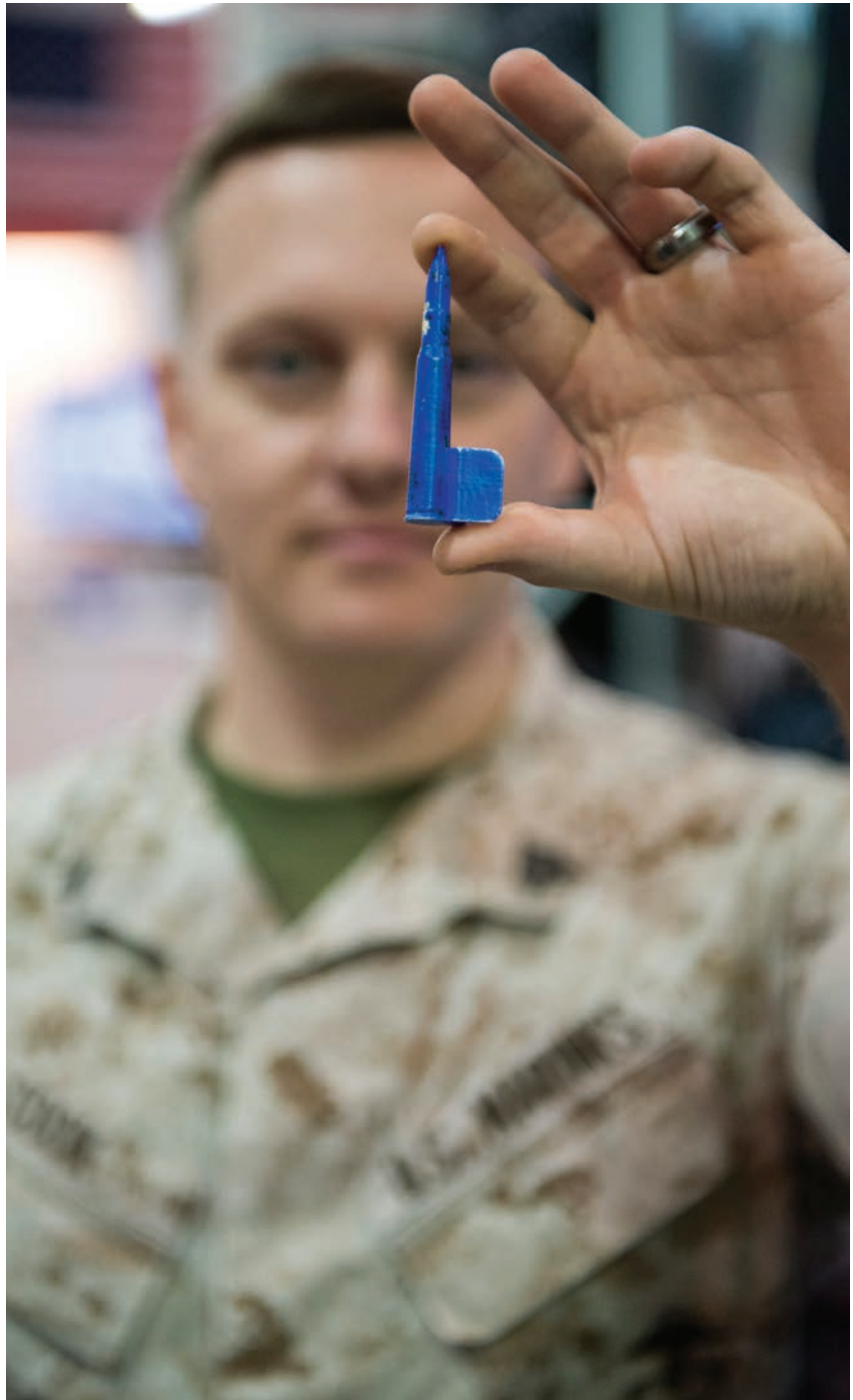
Marine Sgt. Stephen Cook, a legal service specialist with Headquarters Marine Corps, holds up a water cooler spigot in the shape of a rifle round that he printed using additive manufacturing to replace one that had broken at his office during the Modern Day Marine Expo at Marine Corps Base Quantico, Va., Sept. 28, 2016. Cook is sharing his 3-D printing expertise during an additive manufacturing parts demonstration at the expo, which Naval Sea Systems Command, Naval Aviation Systems Command, Marine Corps Systems Command, the Marine Corps Warfighting Laboratory, and Marine Corps Headquarters, Installations and Logistics Department all collaborated on. (U.S. Navy photo by Dustin Q. Diaz/released)
