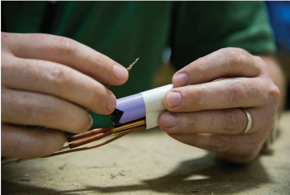
Right: A close up of Kane Ivory, an electrical engineer from Melbourne, Australia, adding thermal couplers and a heating cartridge to a lithium ion cell in West Bethesda, Md., Aug. 29, 2016. (U.S. Navy photo by Dustin Q. Diaz/Released)
