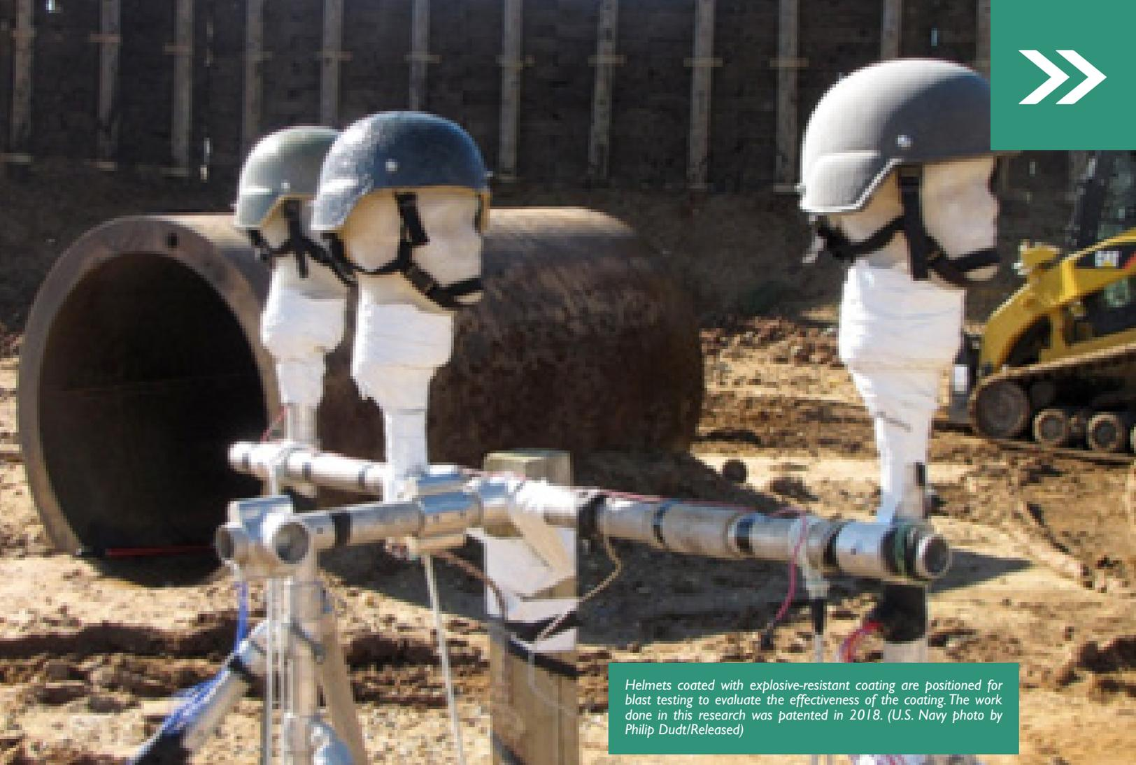
Helmets coated with explosive-resistant coating are positioned for blast testing to evaluate the effectiveness of the coating. The work done in this research was patented in 2018. (U.S. Navy photo by Philip Dudt/Released)
