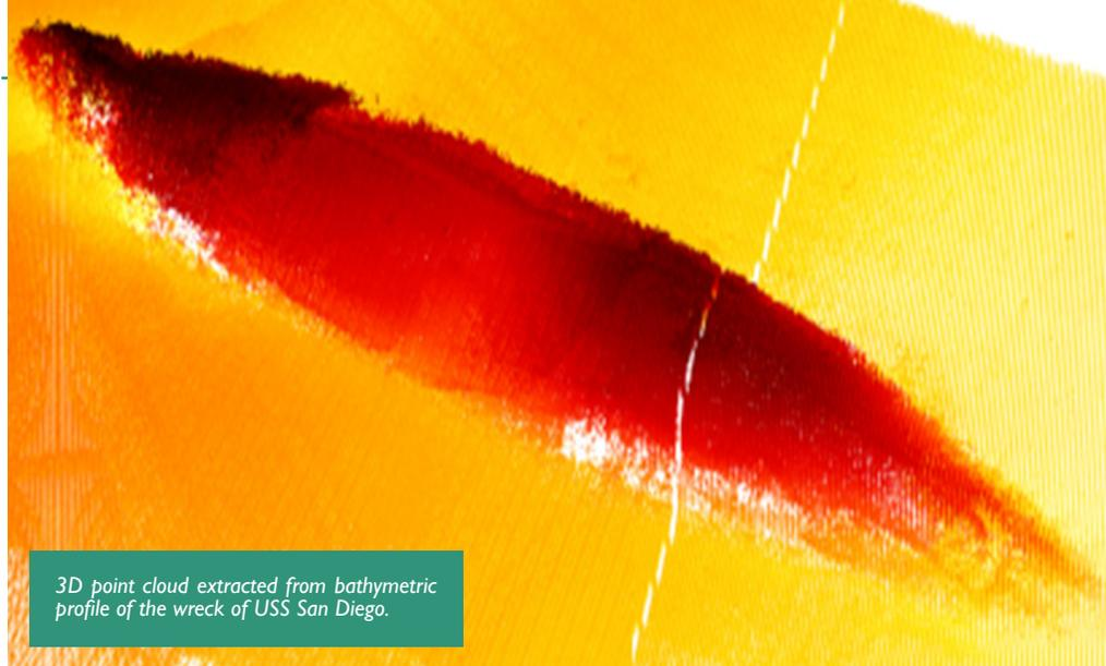
3D point cloud extracted from bathymetric profile of the wreck of USS San Diego.
