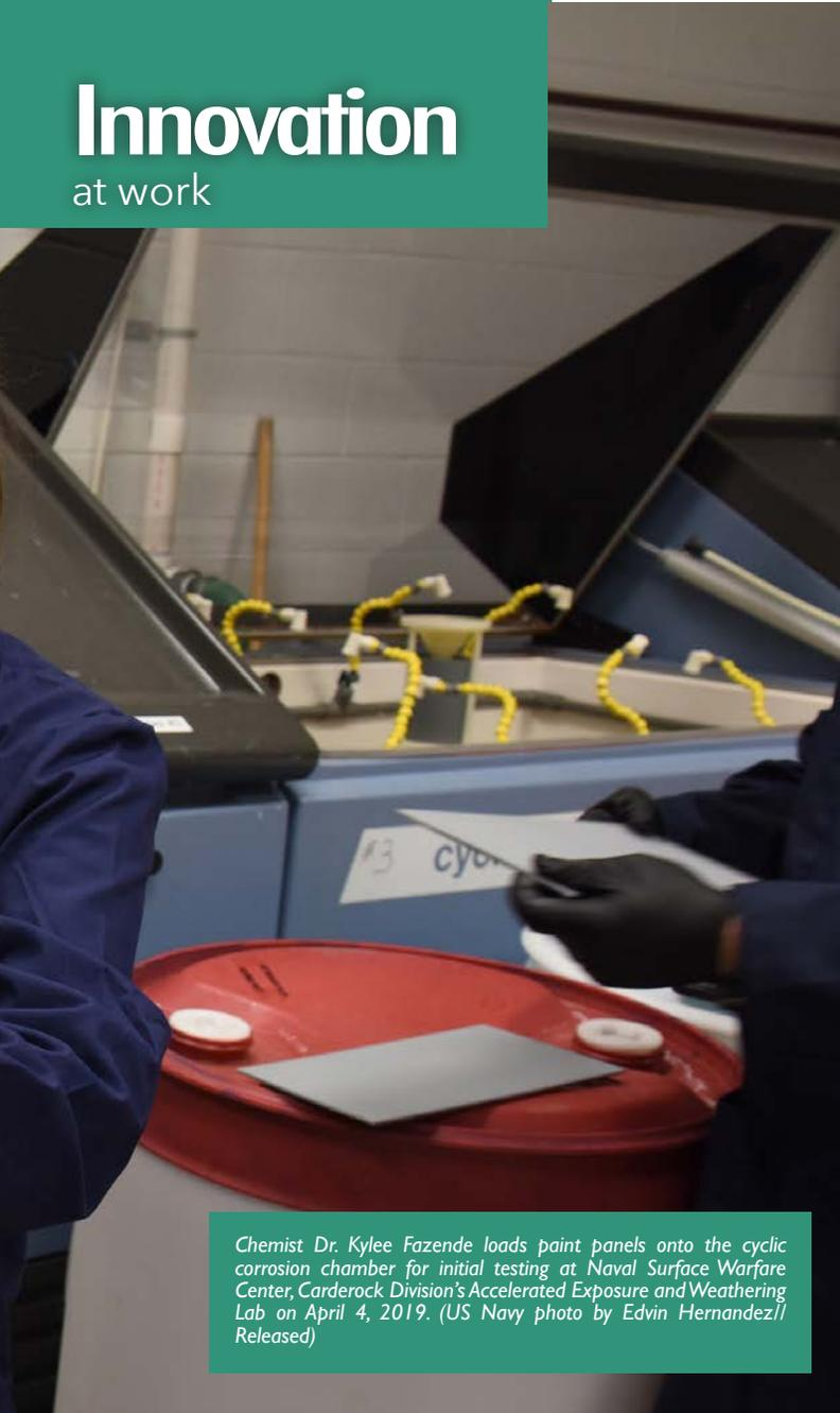
Chemist Dr. Kylee Fazende loads paint panels onto the cyclic corrosion chamber for initial testing at Naval Surface Warfare Center, Carderock Division's Accelerated Exposure and Weathering Lab on April 4, 2019. (US Navy photo by Edwin Hernandez//Released)
