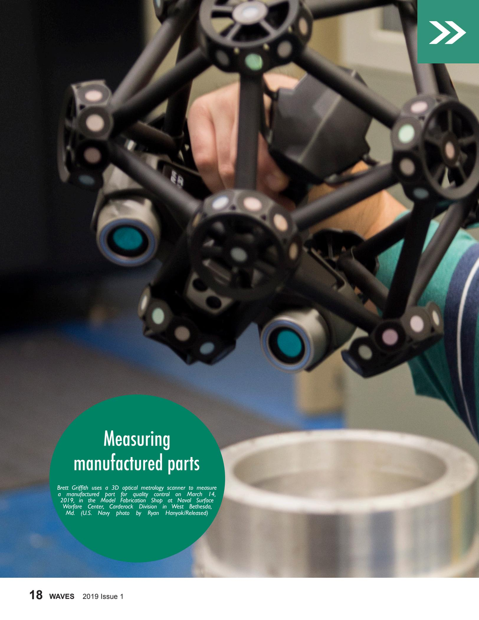
A close-up photograph of a person's hand holding a black 3D optical metrology scanner. The scanner has several colored sensors (green, blue, purple) and is positioned over a large, cylindrical metal part. The background is a blurred industrial setting.
