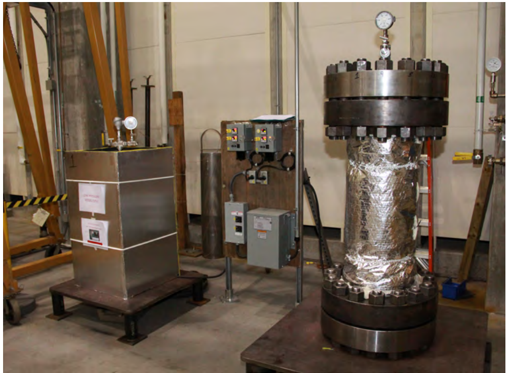
The new Material Conditioning Test Site at NAVSSS has two vertical cylinders - the smaller (left) is rated to 500 psi and the larger (right) at 3,300 psi. Both hold aging fluids such as fresh water, simulated seawater, and hydraulic fluid that can be heated to 200 degrees Fahrenheit. (U.S. Navy photo by Joseph Battista/Released)
