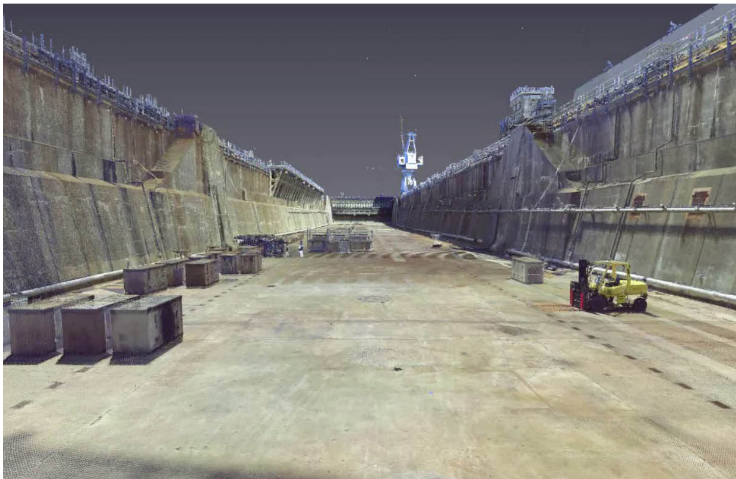
Engineers at Naval Ship Systems Engineering Station create a virtual 3-D model of Norfolk Naval Shipyard's dry dock four June 11-18 to create an advance-planning 3-D layout of the site for determining optimum placement of support services during future dry dockings. (Screenshot provided by Scott Storms/Released)
