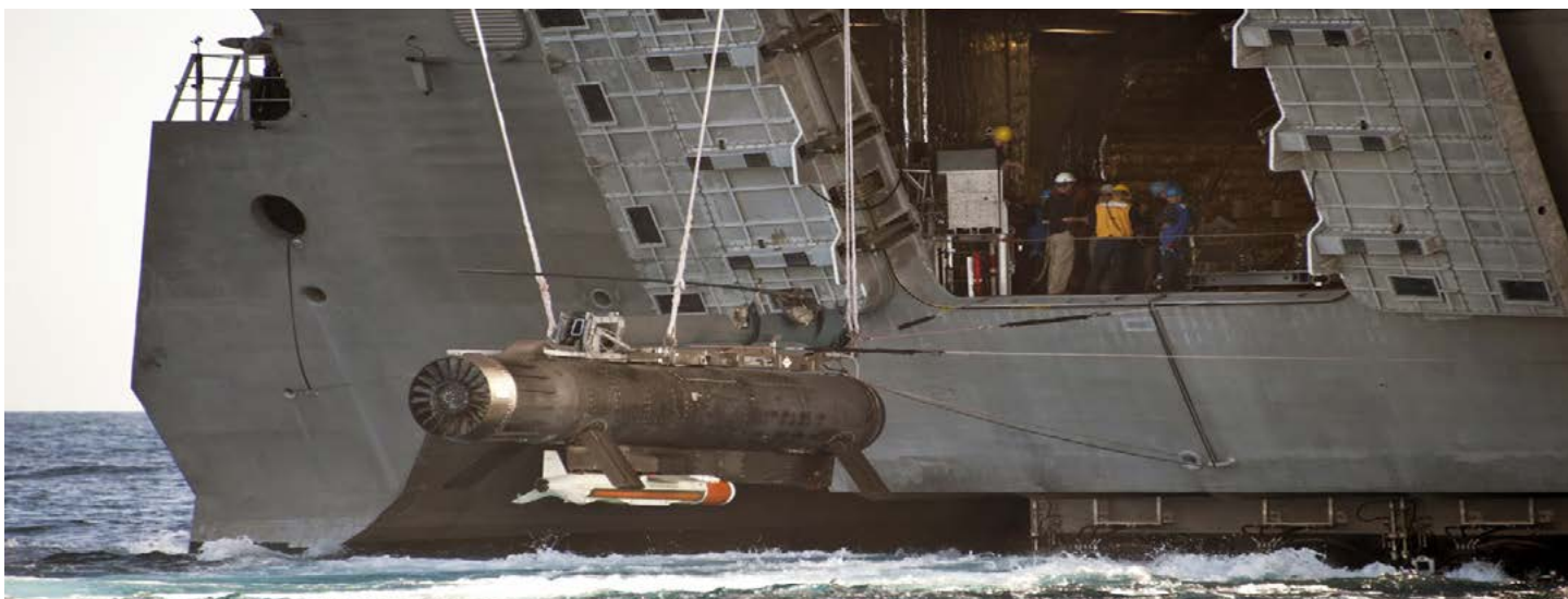
The Remote Multi-Mission Vehicle (RMMV) tows an advanced Variable Depth Sensor (AQS-20A) that supports mine-hunting sensors as part of the Remote Minehunting System (RMS). The RMS is part of the Mine Countermeasures (MCM) Mission Package which provides the primary mine reconnaissance capability for the Navy's Littoral Combat Ship (LCS). (U.S. Navy photo/Released)
