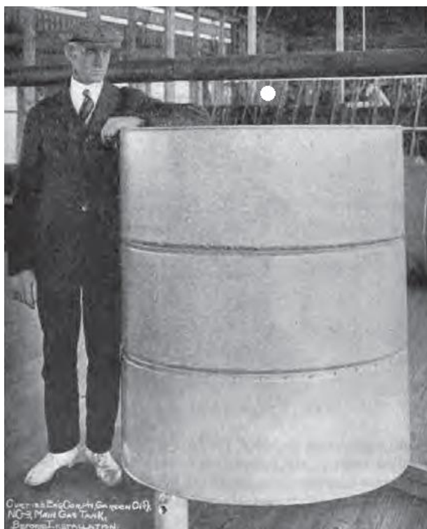
Figure 21. An NC's aluminum fuel tank. The aluminum used in this 200 gallon tank was the first large scale application of aluminum in heavier-than-air aircraft. Its use saved 630 pounds over the equivalent tanks made from steel.
