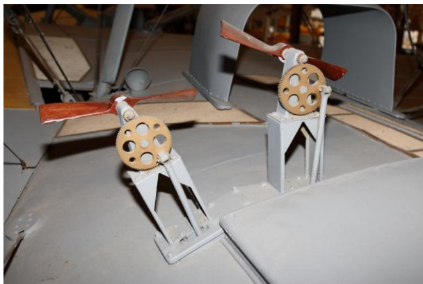
Figure 22. Wind driven fuel pumps. The NC's were equipped with four wind driven pumps (two shown here) to move fuel from the 200 gallon storage tanks in the hull to the gravity tank in the upper wing.
