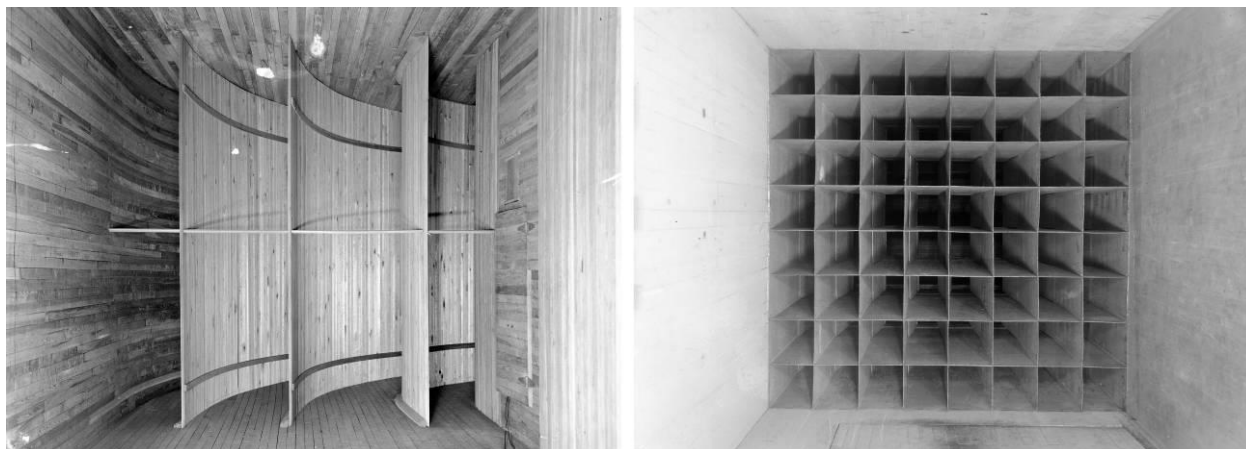
Figure 11. Vertical “splitters” (left) and a honeycomb grid (right) were incorporated into the wind tunnel to enhance flow quality.
