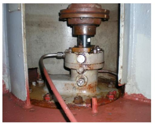
Lube oil service pump before installation of the dry flexible coupling. (U.S. Navy photo by Brett Franks/Released)
